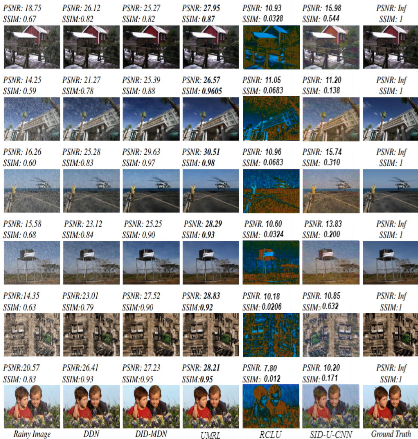
Figure 5.3: De-rained results on synthetic datasets Test-1 and Test-2[23] consisting of different rain levels (low, medium, and heavy) and different directions.
