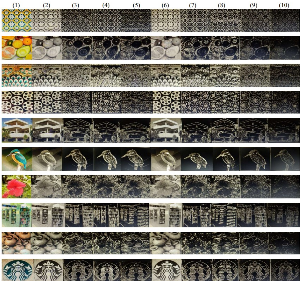
Figure 6.2: (1) Original (2)Gray (3)sobel (4)SobelX (5)SobelY (6)Gaussian blur (7)Prewitt X (8)Prewitt Y (9)Laplacian 8 (10)Laplacian 4
