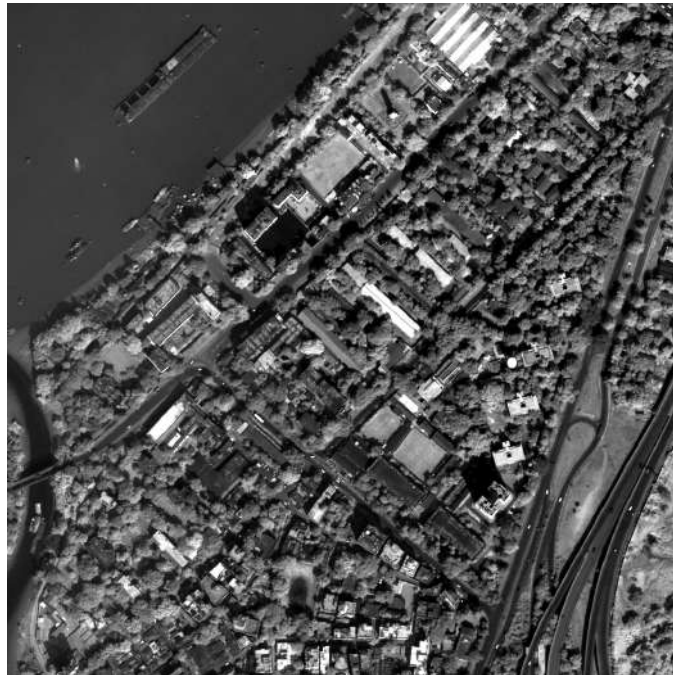
Figure 1.3: Panchromatic (Pan) image with spatial resolution of 0.6m \times 0.6m corresponding to the same geographical area as shown in Fig. 1.1 acquired using Quickbird satellite. The spectral range of Pan sensor is 0.45 - 0.90 \mu m .
