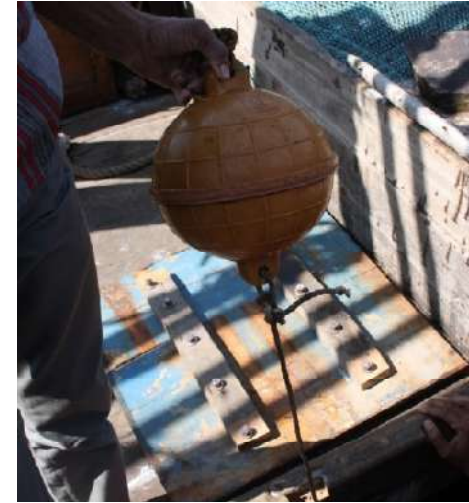
Fig. 13 Float balls used to keep one side of the net floating in the water
