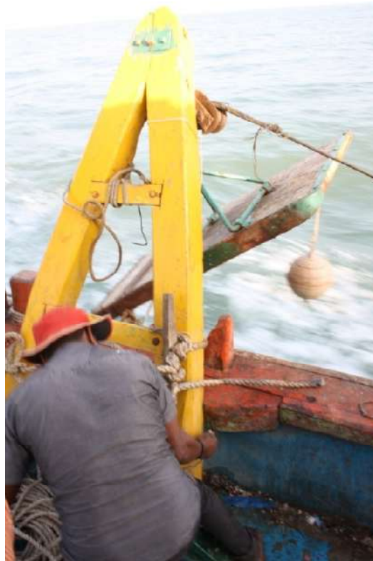
Fig. 17 Fishermen adjusting the angle of the V structure maintain a spread between two wooden boards
