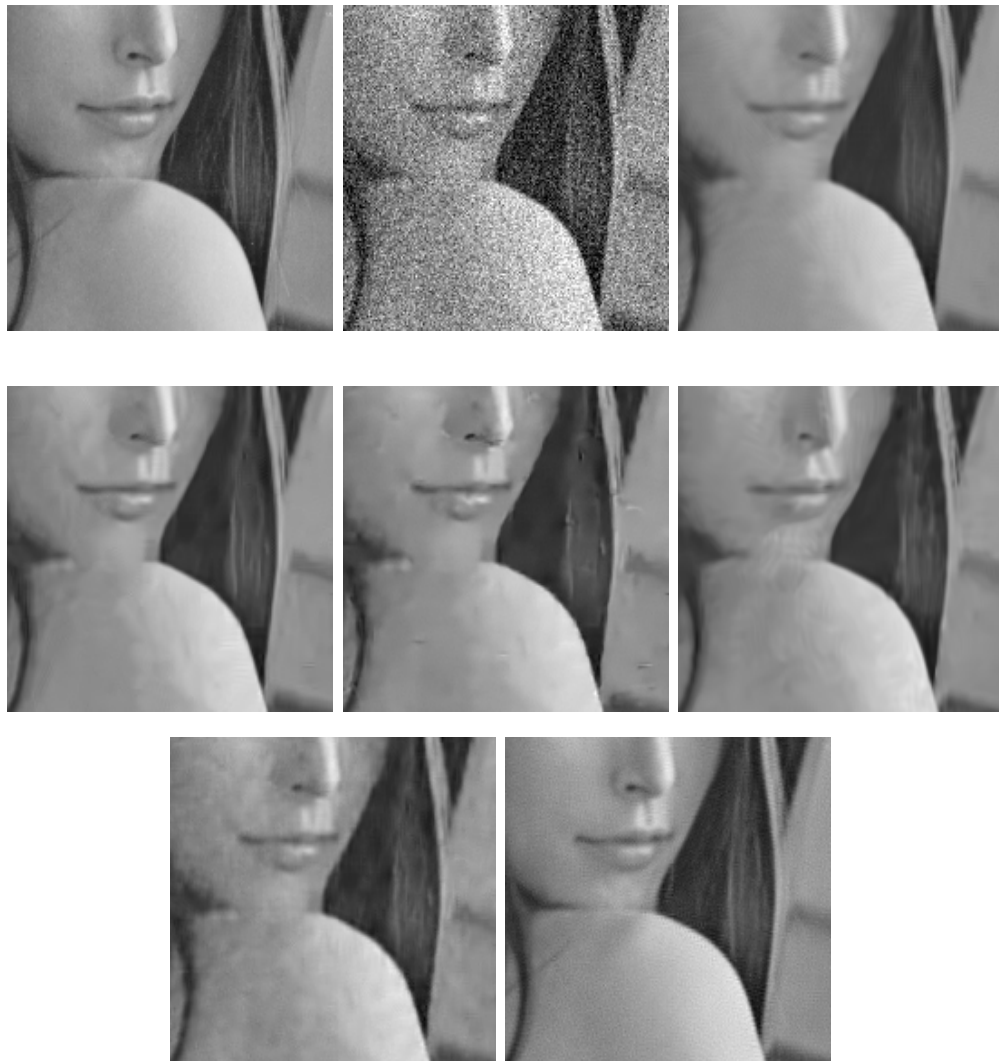
Figure 5.6: Denoising experiment on a portion of ‘Lena’ image. Left to right, top to bottom: Clean image, noisy image ( \sigma = 30 ), LPG-PCA(31.73, 0.847), BM3D(32.38, 0.851), EPLL(31.78, 0.831), CSR(32.36, 0.850), OLPP(31.42, 0.820), 2D-OLPP(33.49, 0.842).
