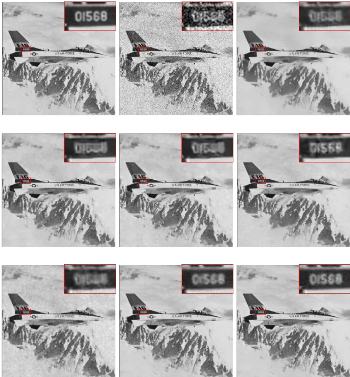
Figure 6.4: Denoising experiment a natural image ('Airplane'), a small part from the image is also zoomed to show the restoration of finer texture. Left to right, top to bottom: Clean image, noisy image ( \sigma = 40 ), LPG-PCA(32.23, 0.894), BM3D(32.55, 0.898), EPLL(32.45, 0.897), CSR(32.68, 0.899), OLPP(32.18, 0.882), 2D-OLPP(32.42, 0.88), 2D-OLPDP(33.46, 0.895).
