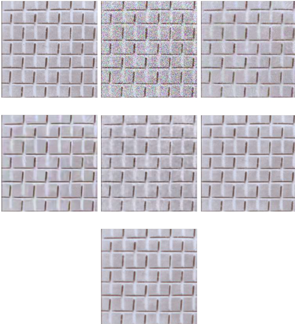
Figure 6.9: Denoising experiment on a color texture image. Left to right, top to bottom: Clean image, noisy image ( \sigma = 50 ), LPG-PCA(25.92, 0.627), BM3D(29.58, 0.815), OLPP(29.25, 0.796), 2D-OLPP(29.89, 0.776), 2D-OLPDP(30.13, 0.787).
