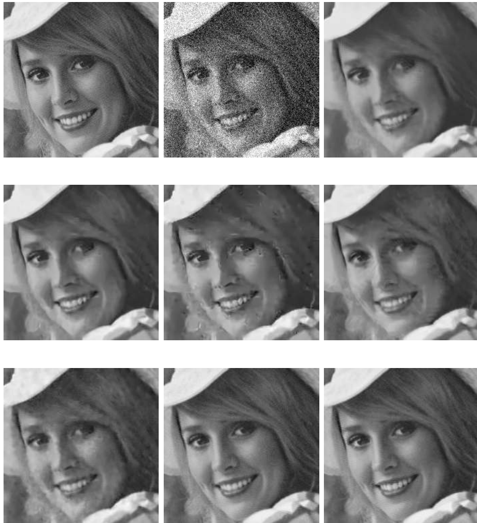
Figure 6.3: Denoising experiment on a part of natural image ('Elaine'). Left to right, top to bottom: Clean image, noisy image ( \sigma = 30 ), LPG-PCA(28.81, 0.678), BM3D(29.17, 0.688), EPLL(28.77, 0.678), CSR(29.79, 0.682), OLPP(28.86, 0.692), 2D-OLPP(31.22, 0.774), 2D-OLPDP(31.50, 0.784).
