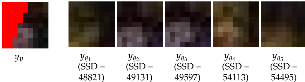
Figure 4.2: Matching patches in exemplar based approaches considering the sum of squared distance (SSD) measure. Here, y_p is the patch selected for inpainting with the missing pixels shown in red color. The patches y_{q_1}, \dots, y_{q_5} are the most similar patches to y_p in terms of SSD. Although y_{q_1} has a smaller value for SSD, we observe y_{q_2} and y_{q_3} to be better sources for filling the missing pixels in y_p . Note that red color indicates region only and not the color pixels.
