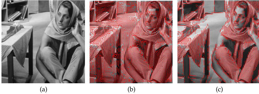
Figure 6.9: Orientation map of Barbara image using a block size of 8 \times 8 . (a) Original Barbara image (size: 512 \times 512 ) (b) orientation map [35] (c) corrected orientation map.
