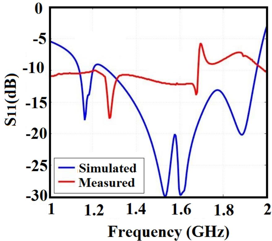
Figure 4.10: Simulated and measured return loss of dual-band CP RDRA for L5 and L1-bands [1]
