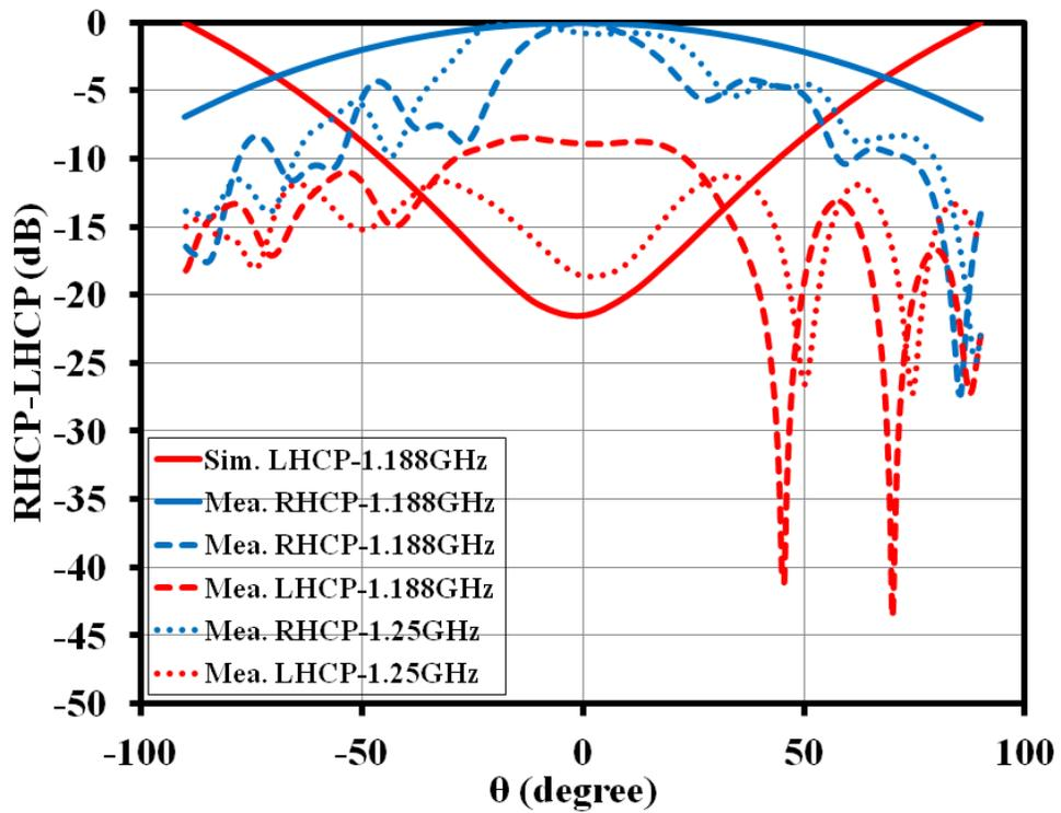
Figure 5.41: Simulated and measured RHCP-LHCP far field radiation patterns for L5-band at  $\phi=0^\circ$  [6]
