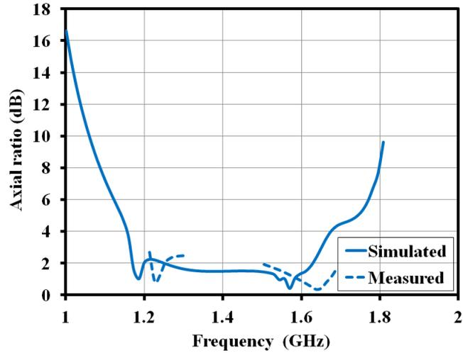
Figure 4.15: Simulated and measured axial ratio at L5 and L1-bands of dual-band RDRA
