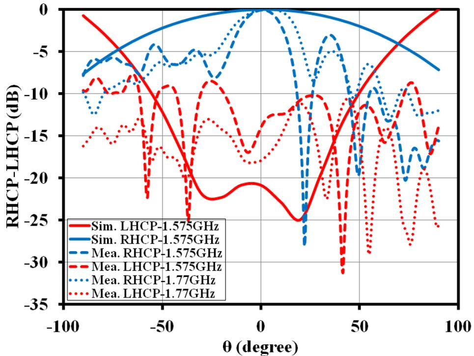
Figure 5.37: Simulated and measured RHCP-LHCP far field radiation patterns for L1-band at  $\phi=90^\circ$  [6]
