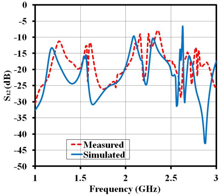
Figure 3.17: Simulated and measured  $S_{12}$  of tri-band RDRA (two port) [1]
