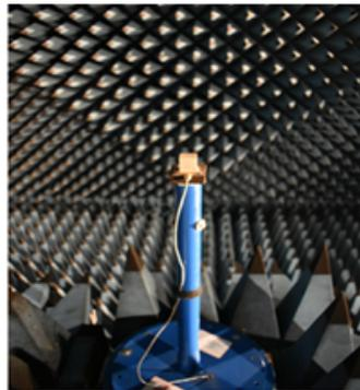
Figure 5.18: Photograph of fabricated single-band RDRA for test and measurement in the anechoic chamber
