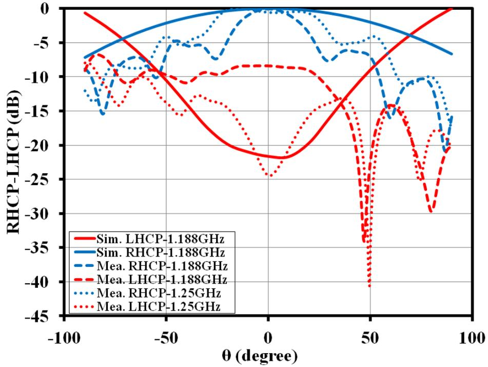
Figure 5.42: Simulated and measured RHCP-LHCP far field radiation patterns for L5-band at  $\phi=45^\circ$  [6]
