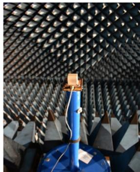
Figure 3.14: Fabricated tri-band RDRA in anechoic chamber [8]
