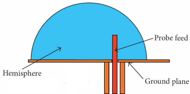
Figure 2.2: HDRA with probe-fed [1]
