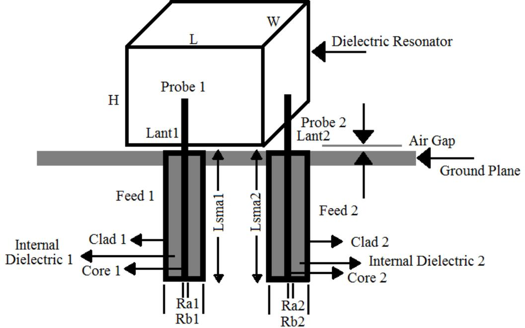
Figure B.1: Geometry of two port single- and dual-band CP RDRAs
