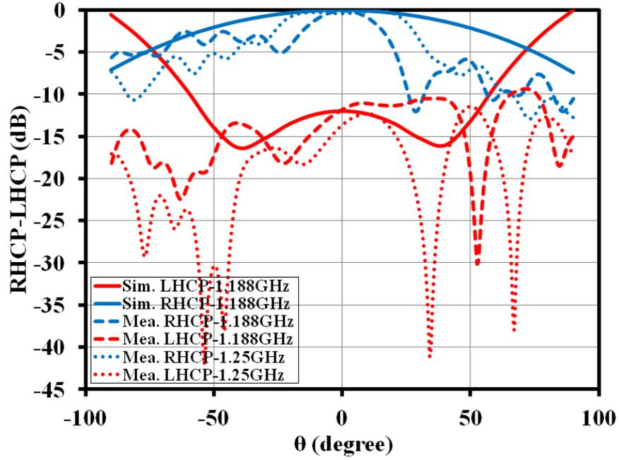
Figure 3.35: Simulated and measured RHCP-LHCP radiation patterns at L5-band for  $\phi=90^\circ$  of tri-band RDRA (single port) [8]
