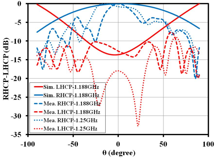
Figure 3.29: Simulated and measured RHCP-LHCP radiation patterns at L5-band for  $\phi=0^\circ$  of tri-band RDRA (single port) [8]
