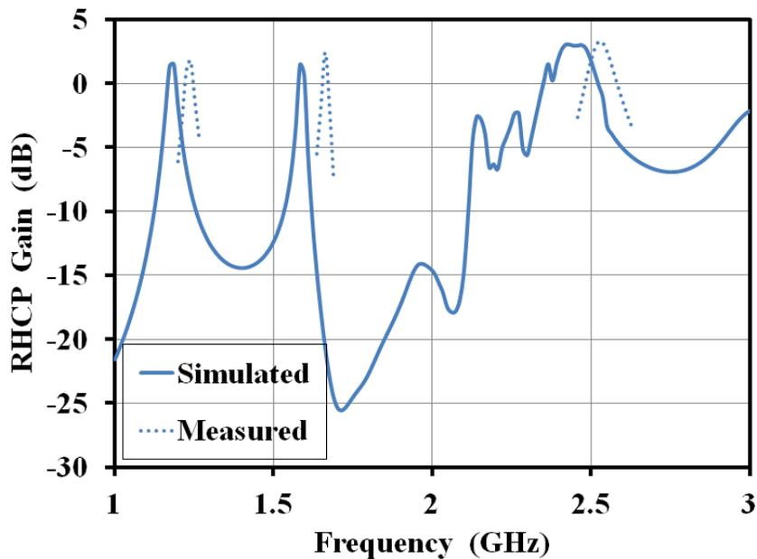
Figure 3.38: Simulated and measured RHCP gain of tri-band RDRA (single port)
