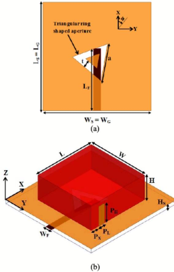
Figure 2.25: (a) Top view (b) 3-D geometry of dual-band CP RDRA [35]
