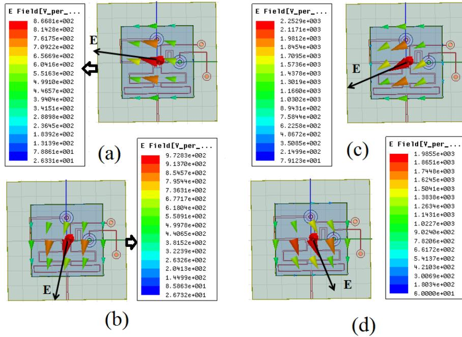
Figure 4.7: Electric field distribution of dual-band RDRA (a) 1.176 GHz with respect to  $0^\circ$  (b) 1.176 GHz with respect to  $90^\circ$  (c) 1.575 GHz with respect to  $0^\circ$  (d) 1.575 GHz with respect to  $90^\circ$
