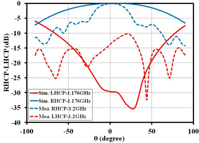
Figure 3.25: Simulated and measured RHCP-LHCP radiation patterns of tri-band RDRA at L5-band for  $\phi=90^\circ$  [1]
