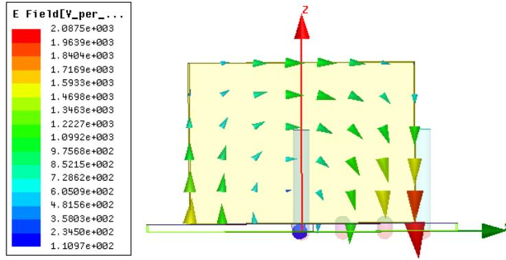
Figure 5.6: Electric field distribution of  $TE_{111}^y$  mode at 2.49 GHz
