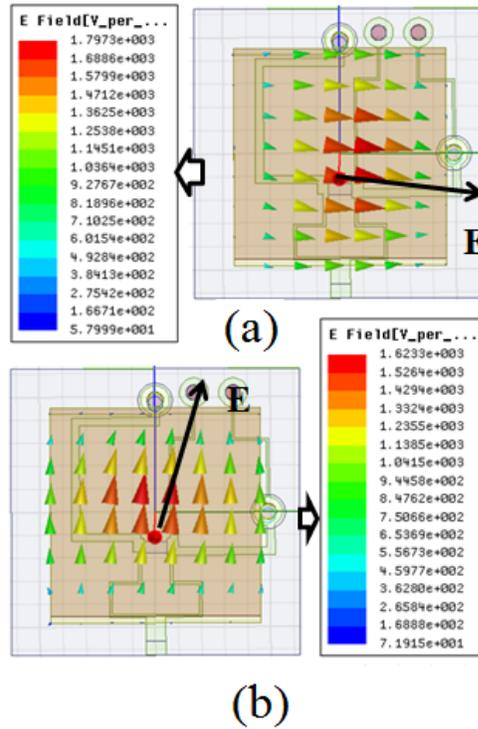
Figure 5.7: (a) Electric field distribution at 2.49 GHz with respect to  $0^\circ$ , and (b) electric field distribution at 2.49 GHz with respect to  $90^\circ$
