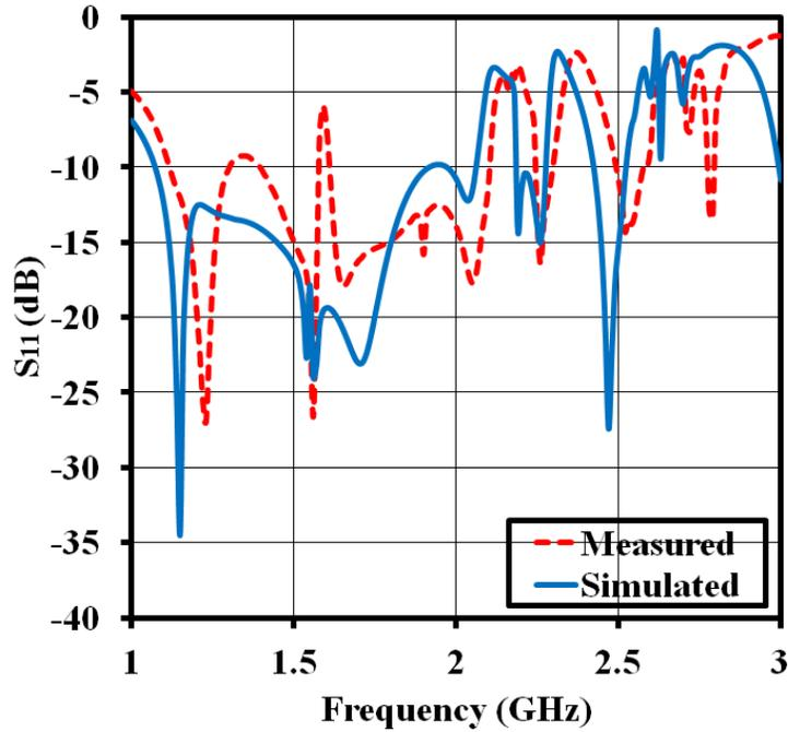
Figure 3.15: Simulated and measured  $S_{11}$  of tri-band RDRA (two port) [1]
