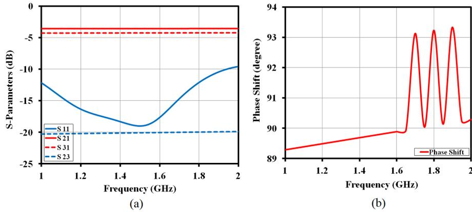
Figure 4.5: Results of feed network (a) S-parameters of dual section WPD with  $90^\circ$  phase shifter (b) phase shift of dual section WPD with  $90^\circ$  phase shifter
