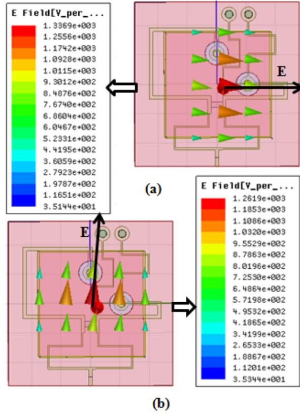
Figure 5.16: (a) Electric field distribution at 1.575 GHz with respect to  $0^\circ$ , and (b) electric field distribution at 1.575 GHz with respect to  $90^\circ$  [6]
