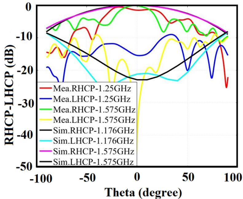
Figure 4.11: Simulated and measured RHCP-LHCP radiation patterns at L5 and L1-band of dual-band DRA for  $\phi=0^\circ$  [1]
