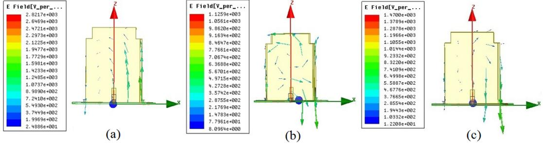
Figure 3.5: Electric field distribution of tri-band RDRA
