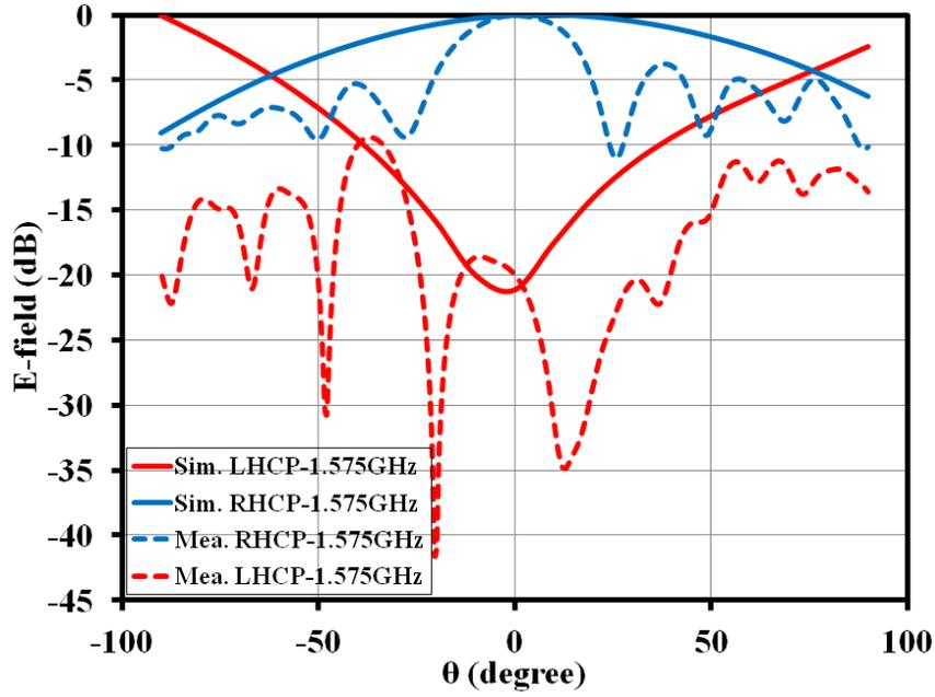
Figure 3.33: Simulated and measured RHCP-LHCP radiation patterns at L1-band for  $\phi=45^\circ$  of tri-band RDRA (single port) [8]
