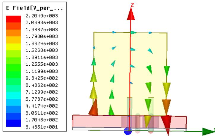
Figure 5.15: Electric field distribution of  $TE_{111}^y$  mode at 1.575 GHz [6]
