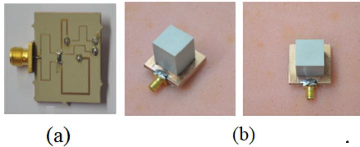
Figure 5.17: Photograph of (a) bottom view (b) 3-D geometries views of fabricated single-band RDRA [6]
