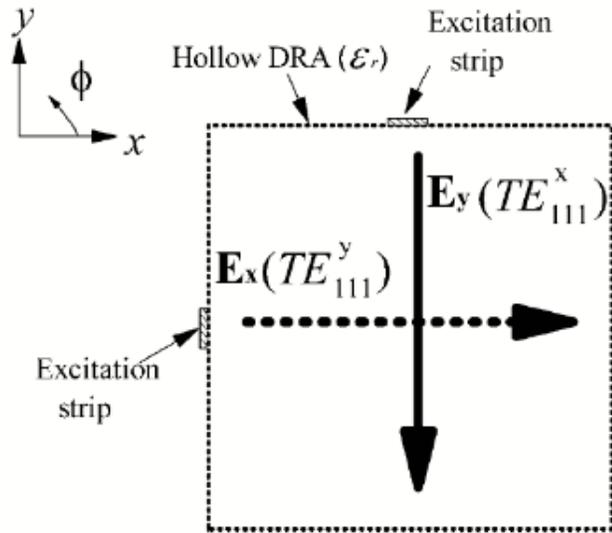
Figure 2.31: Electric fields of CP hollow RDRA [45]
