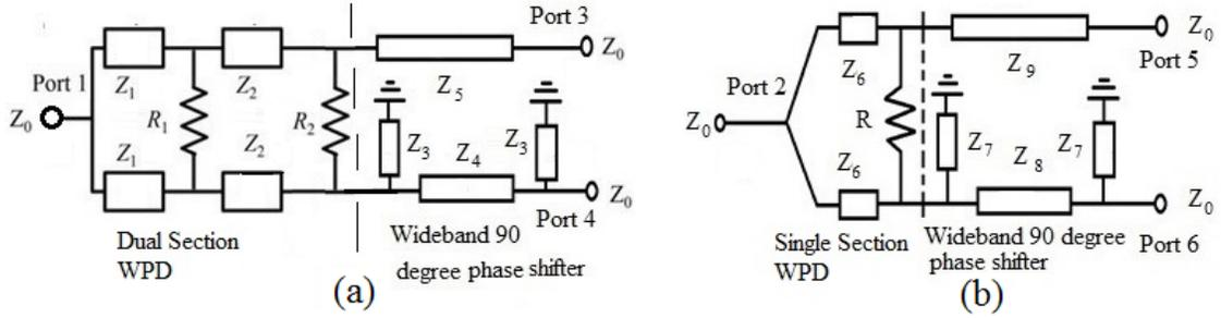
Figure 3.2: Feed networks of triband staired RDRA (a) configuration of dual section WPD with wideband  $90^\circ$  phase shifter (b) configuration of single-section WPD with wideband  $90^\circ$  phase shifter [1, 5, 6, 7]
