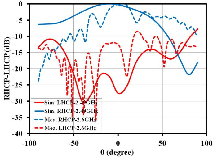
Figure 3.27: Simulated and measured RHCP-LHCP radiation patterns of tri-band RDRA at S-band for  $\phi=90^\circ$  [1]
