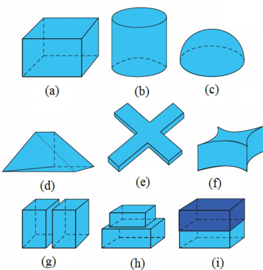
Figure 2.1: Different radiating geometries of DRAs [1]
