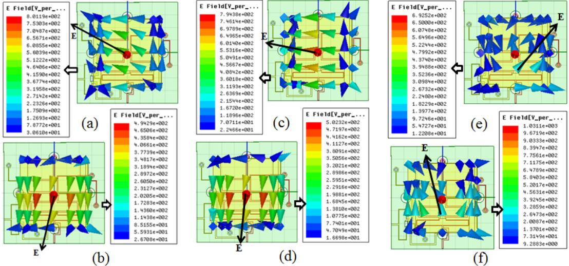
Figure 3.6: Electric field distribution of tri-band RDRA (a) 1.176 GHz with respect to  $0^\circ$  (b) 1.176 GHz with respect to  $90^\circ$  (c) 1.575 GHz with respect to  $0^\circ$  (d) 1.575 GHz with respect to  $90^\circ$  (e) 2.49 GHz with respect to  $0^\circ$  (f) 2.49 GHz with respect to  $90^\circ$  [1]
