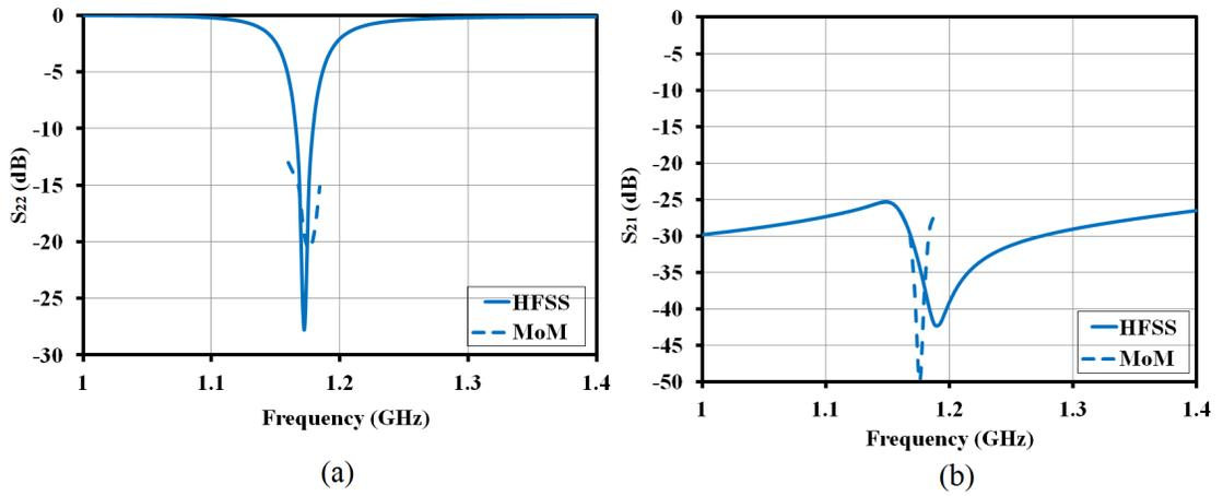
Figure 6.11: (a)  $S_{22}$  and (b)  $S_{21}$  of single-band RDRA using reference [3] and MoM
