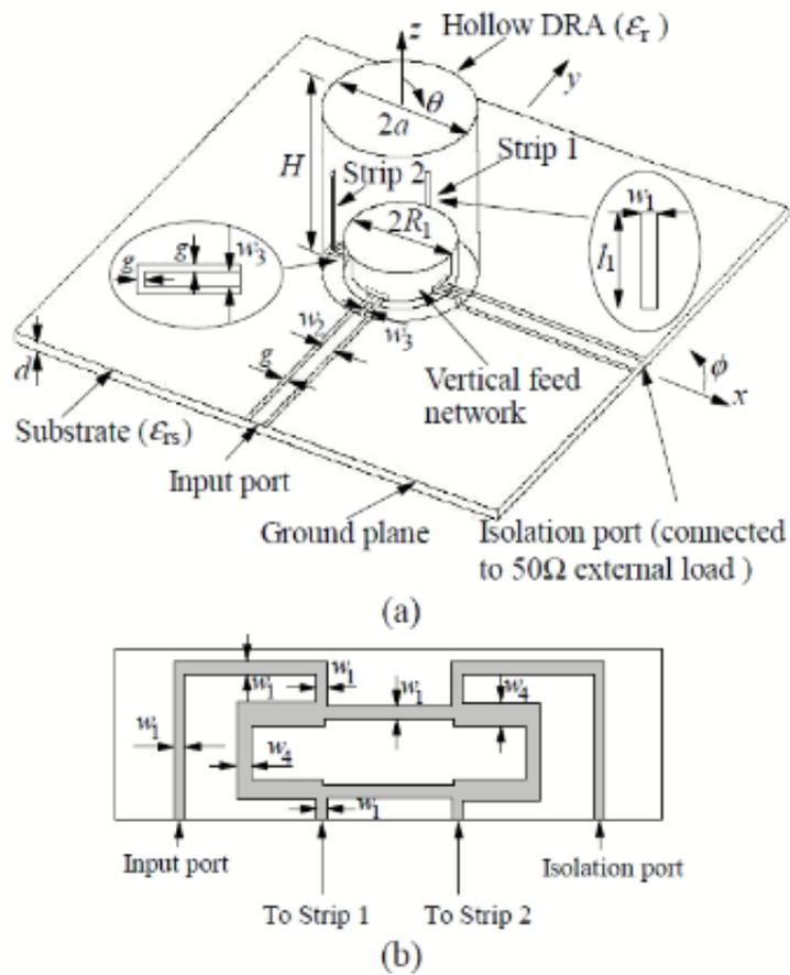
Figure 2.32: (a) 3-D view of CP hollow CDRA with embedded vertical feed network (b) layout of excitation [48]
