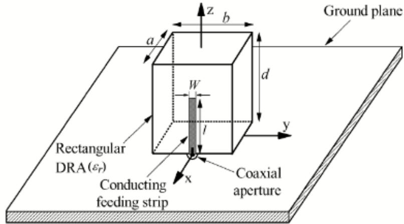
Figure 2.7: Geometry of the strip-fed RDRA [7]
