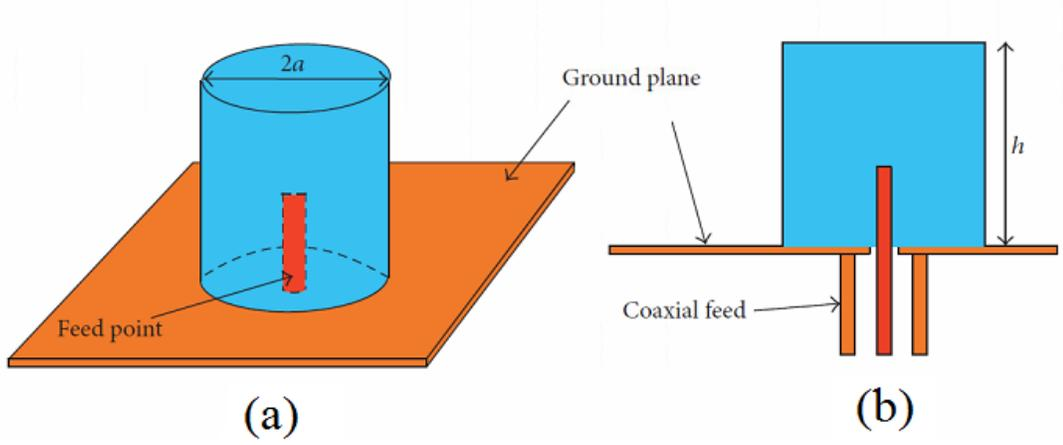
Figure 2.3: (a) 3-D cross-sectional view of CDRA (b) probe-fed CDRA [1]
