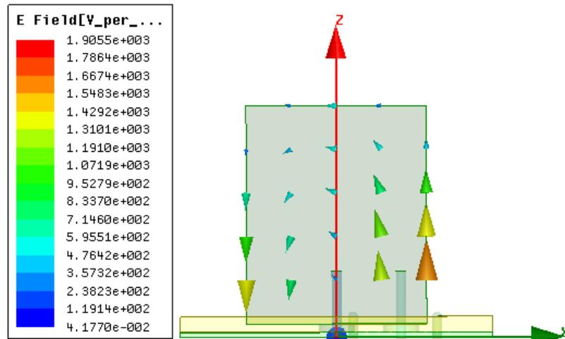
Figure 5.24: Electric field distribution of  $TE_{111}^y$  mode at 1.176 GHz [6]
