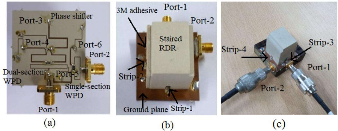
Figure 3.7: Photograph of fabricated triband RDRA (a) bottom view (b) top view (c) side view [1]
