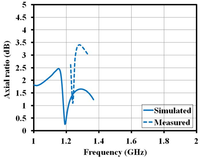
Figure 5.45: Simulated and measured axial ratio of single-band RDRA [6]
