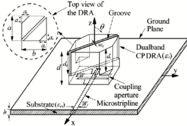
Figure 2.20: 3-D geometry of dual-band RDRA [28]
