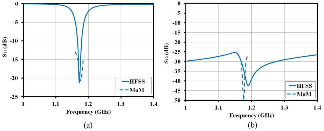
Figure 6.10: (a)  $S_{11}$  and (b)  $S_{12}$  of single-band RDRA using reference [3] and MoM
