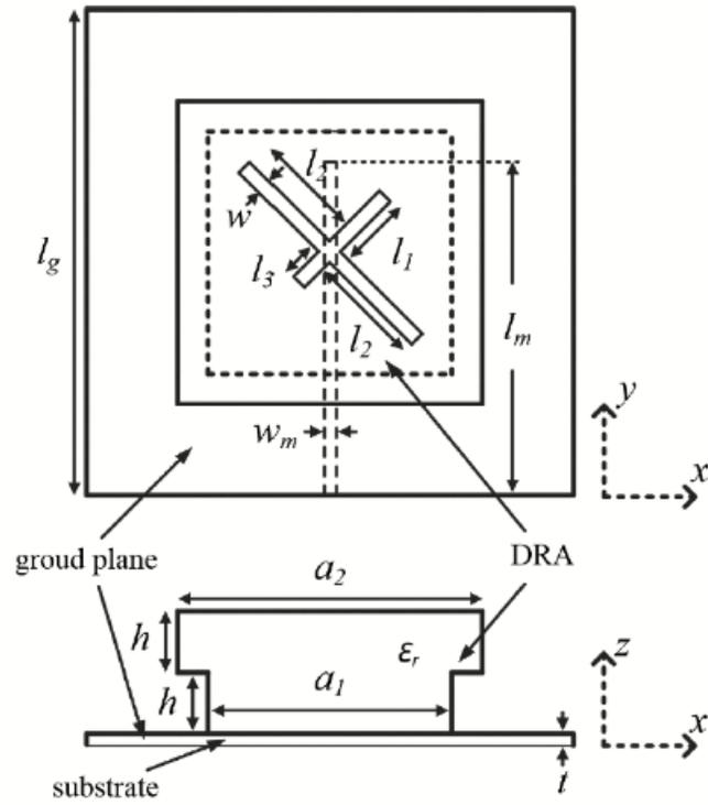
Figure 2.22: Structure of wide dual-band CP stacked RDRA [29]
