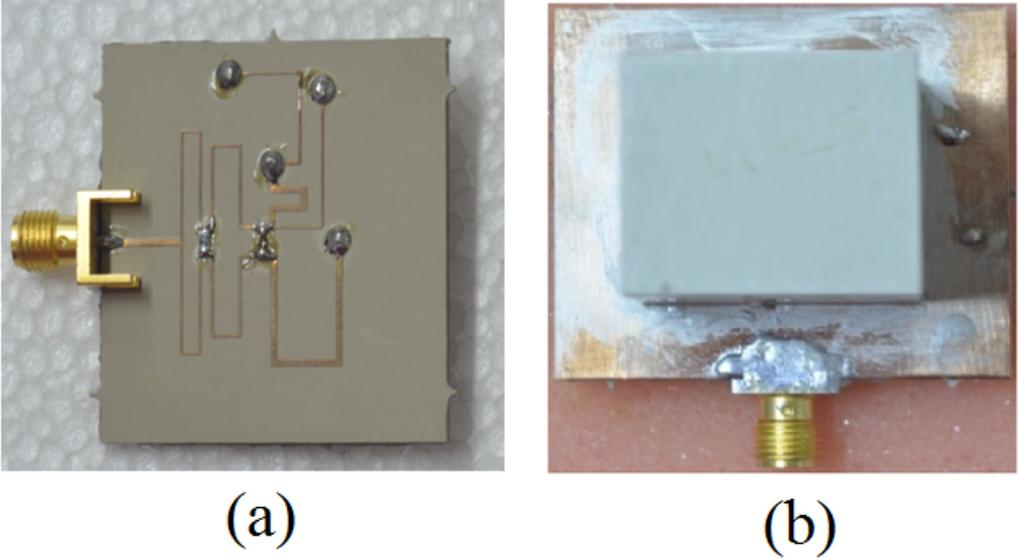
Figure 4.8: Fabricated dual-band RDRA (a) bottom view (b) top view
