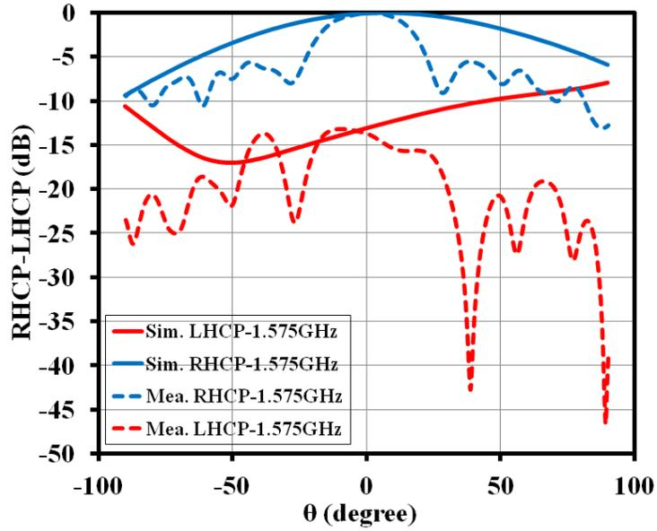
Figure 3.20: Simulated and measured RHCP-LHCP radiation patterns of tri-band RDRA at L1-band for  $\phi=0^\circ$  [1]
