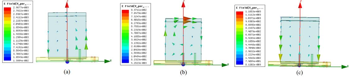
Figure 3.11: Electric field distribution of tri-band RDRA (a)  $TE_{111}^y$  mode at 1.176 GHz (b)  $TE_{113}^y$  mode at 1.575 GHz (c)  $TE_{112}^y$  mode at 2.49 GHz [8]
