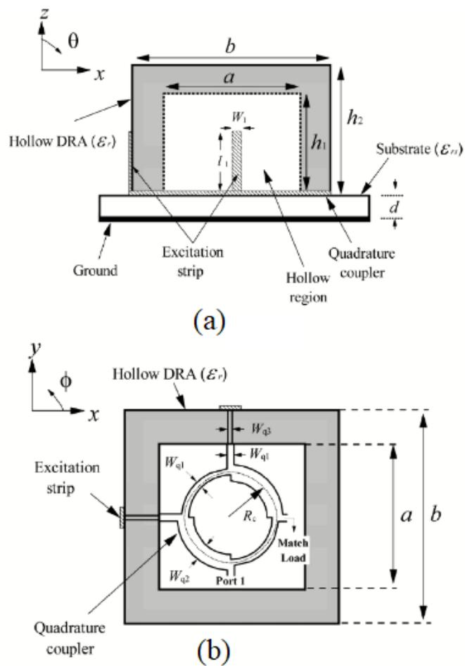
Figure 2.30: (a) Front view (b) top view of CP hollow RDRA with an underlaid quadrature coupler [45]
