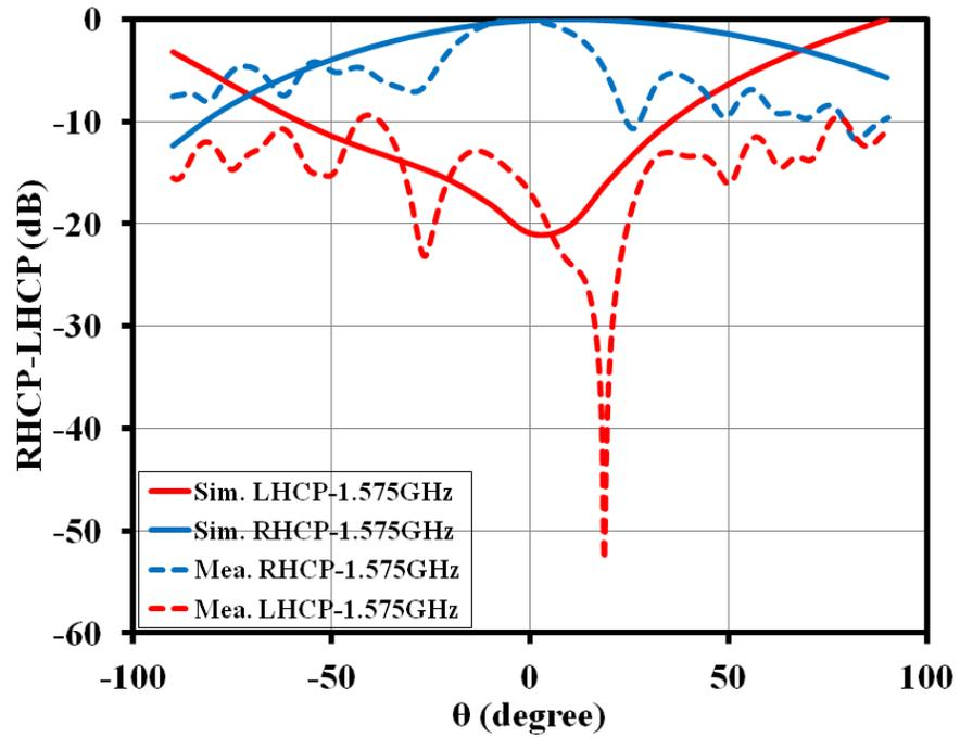
Figure 3.30: Simulated and measured RHCP-LHCP radiation patterns at L1-band for  $\phi=0^\circ$  of tri-band RDRA (single port) [8]
