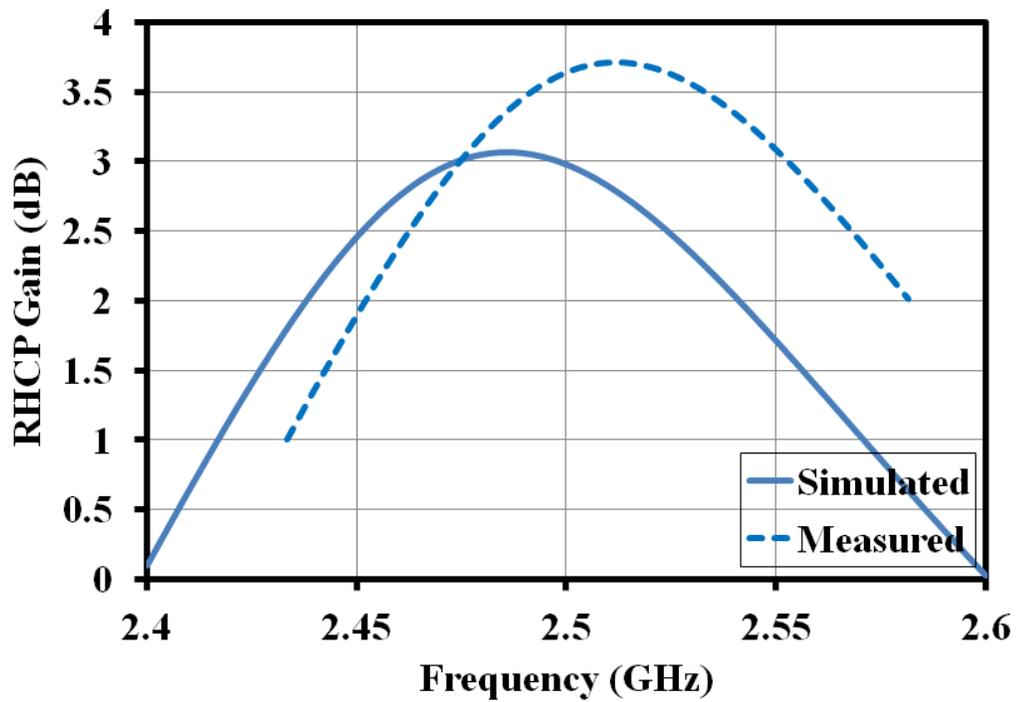
Figure 5.32: Simulated and measured RHCP gain of single-band RDRA
