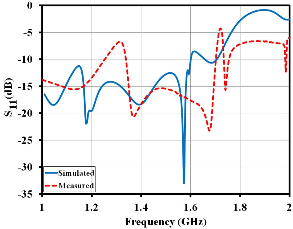
Figure 5.40: Simulated and measured  $S_{11}$  of single-band RDRA [6]
