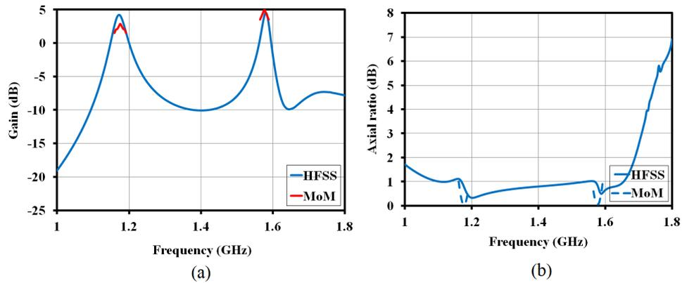
Figure 6.7: (a) Gain and (b) axial ratio of dual-band RDRA using reference [3] and MoM
