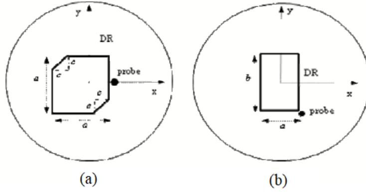
Figure 2.33: (a) Top view of structure-1 and (b) top view of structure-2 of modified CP RDRA [50]
