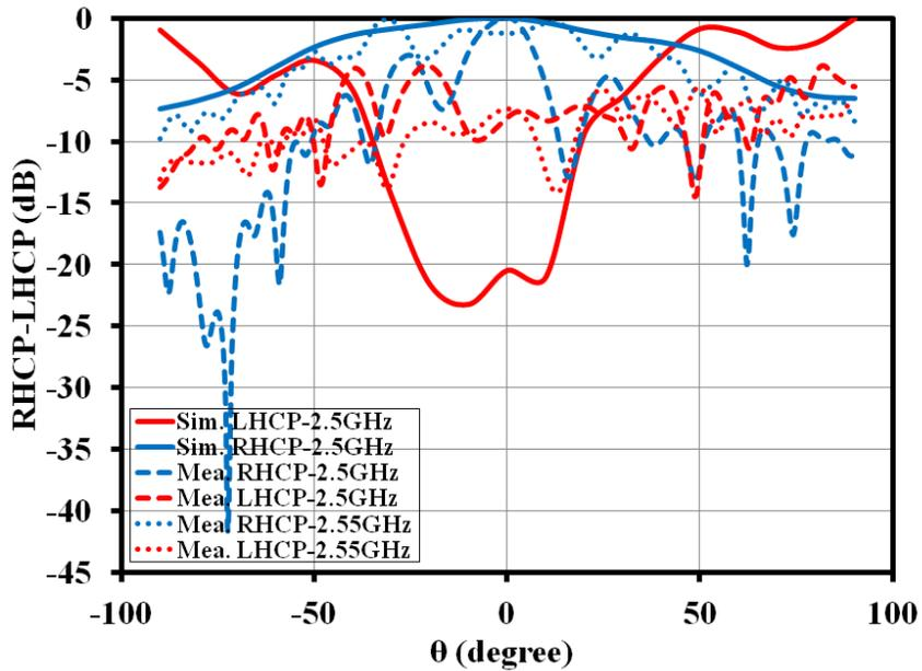
Figure 3.37: Simulated and measured RHCP-LHCP radiation patterns at S-band for  $\phi=90^\circ$  of tri-band RDRA (single port) [8]
