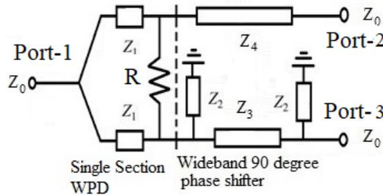
Figure 5.22: Feed network of WPD with wide-band  $90^\circ$  phase shifter [1, 3, 4]
