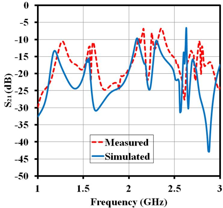
Figure 3.18: Simulated and measured  $S_{21}$  of tri-band RDRA (two port) [1]
