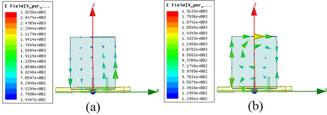
Figure 4.6: Electric field distribution of dual-band RDRA (a)  $TE_{111}^y$  mode at 1.176 GHz (b)  $TE_{113}^y$  mode at 1.575 GHz [1]
