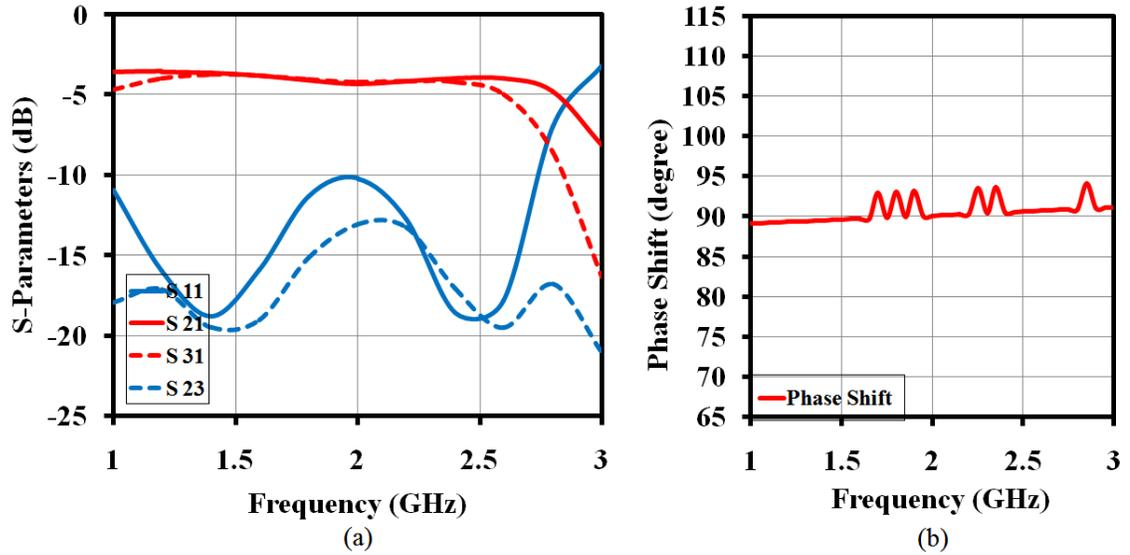
Figure 3.10: (a)  $S_{11}$ ,  $S_{21}$ ,  $S_{31}$  and  $S_{23}$  (b) phase shift of tri-section WPD with wide-band 90° phase shifter [8]
