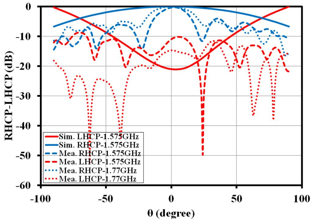
Figure 5.35: Simulated and measured RHCP-LHCP far field radiation patterns for L1-band at  $\phi=0^\circ$  [6]
