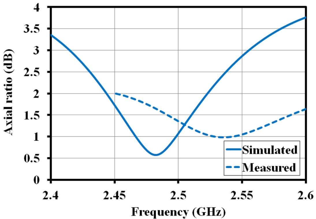
Figure 5.33: Simulated and measured axial ratio of single-band RDRA
