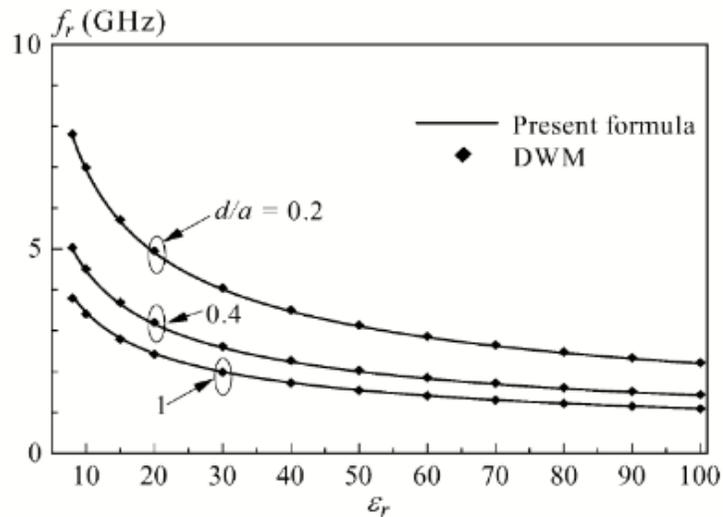
Figure 2.8: The resonance frequency of RDRA as function of  $\epsilon_r$  for  $d/a=0.2, 0.4$  and  $1$ :  $a=20$  mm and  $b=12$  mm [7]
