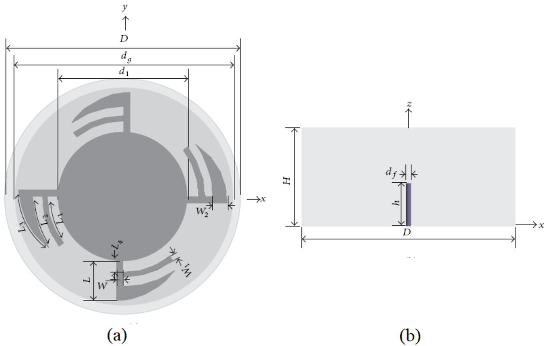
Figure 2.13: Geometry of tri-band CP DRA with top-loaded alford loop (a) top view (b) side view [13]
