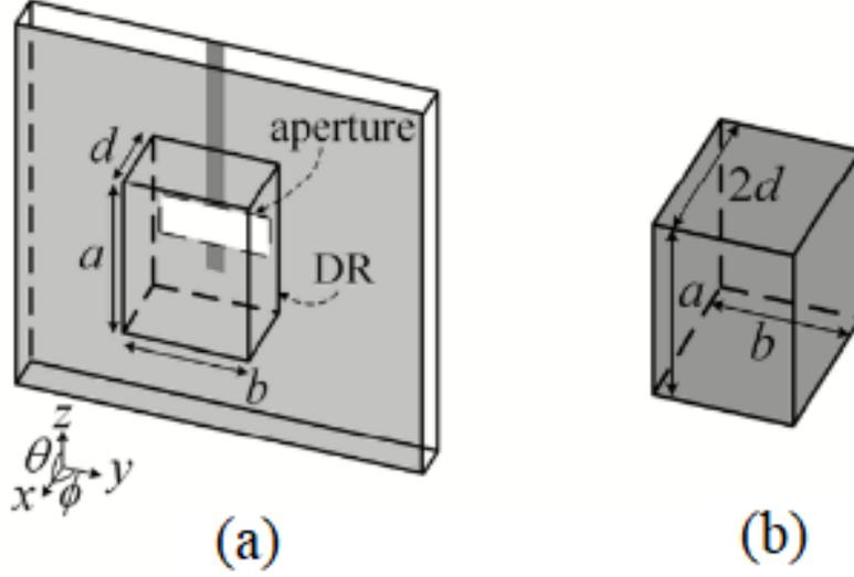
Figure 2.6: (a) Dielectric resonator on ground plane (b) equivalent dielectric resonator in free-space [6]
