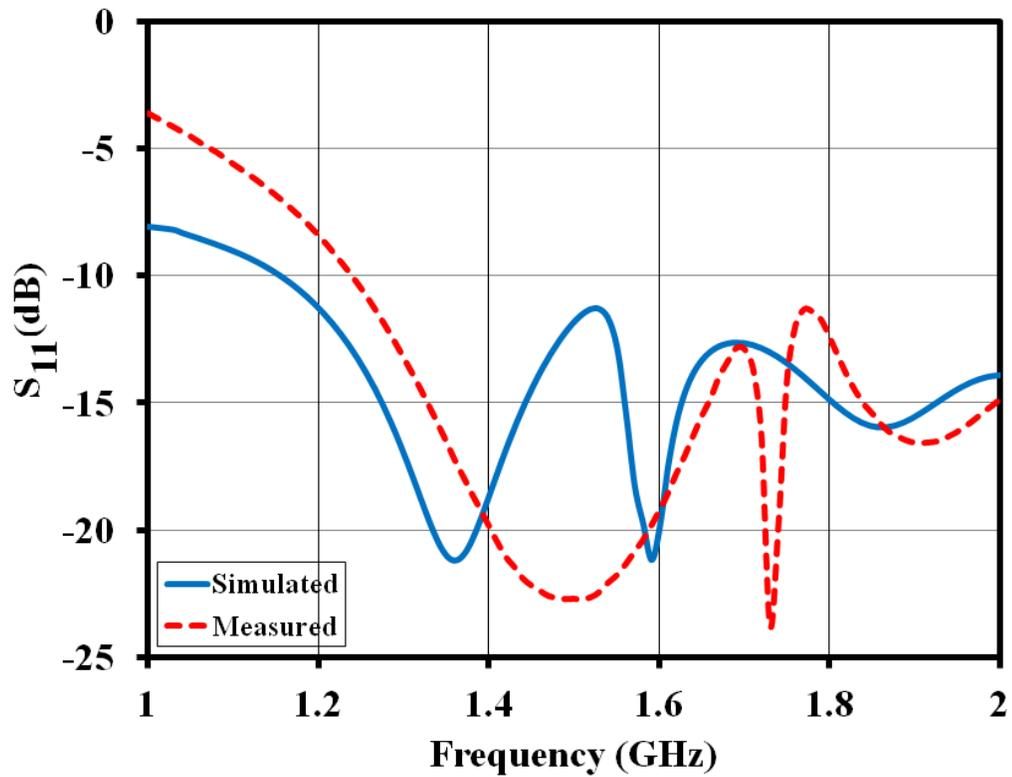
Figure 5.34: Simulated and measured  $S_{11}$  of single-band RDRA [6]
