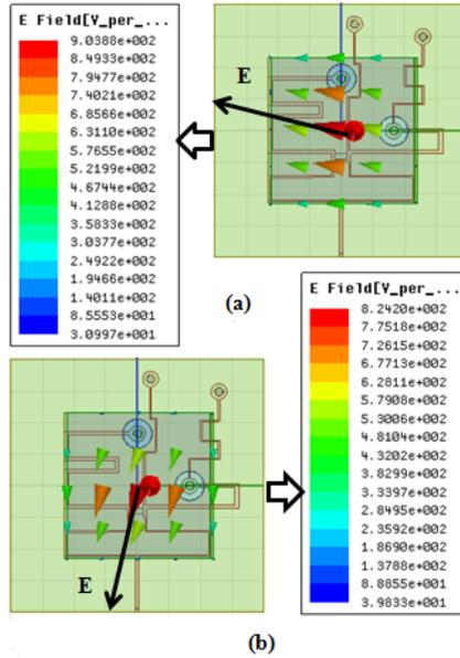
Figure 5.25: (a) Electric field distribution at 1.176 GHz with respect to  $0^\circ$ , and (b) electric field distribution at 1.176 GHz with respect to  $90^\circ$  [6]
