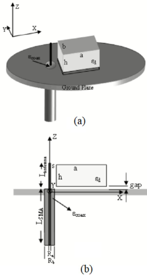
Figure 2.37: (a) 3-D Geometry (b) side view of probe-fed RDRA on finite ground plane [63]
