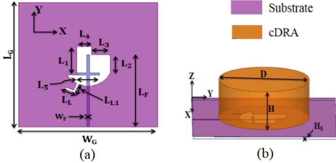
Figure 2.14: Geometry of quad-band quad-sense CP CDRA (a) top view without cylindrical DR (b) isometric view [14]
