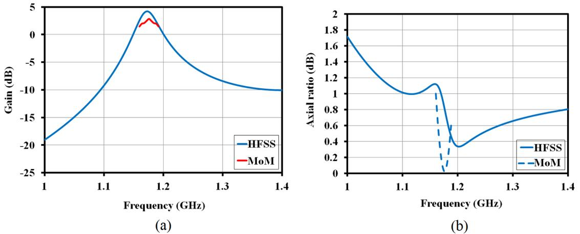
Figure 6.12: (a) Gain and (b) axial ratio of single-band RDRA using reference [3] and MoM
