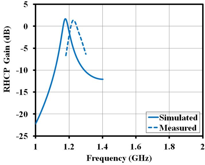
Figure 5.44: Simulated and measured RHCP gain of single-band RDRA [6]
