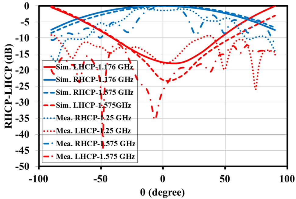
Figure 4.12: Simulated and measured RHCP-LHCP radiation patterns at L5 and L1-band of dual-band DRA for  $\phi=45^\circ$
