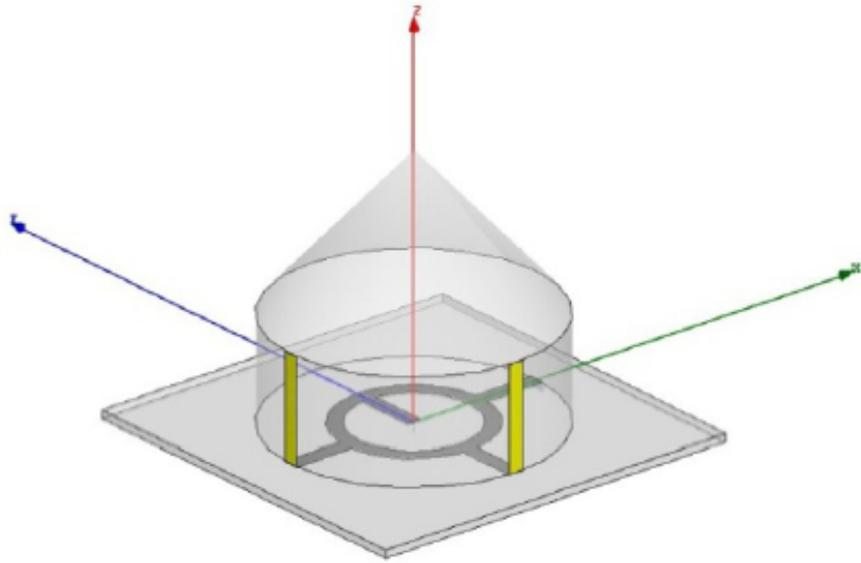
Figure 2.12: 3-D geometry of all GPS bands CP DRA with hybrid ring excitation [12]
