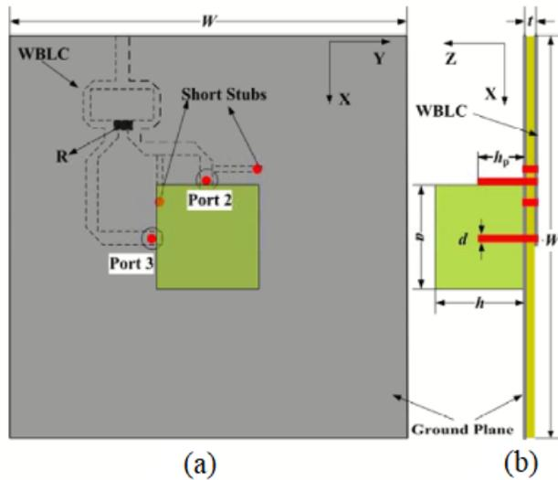
Figure 2.28: (a) Top view (b) side view of CP DRA with wide-band feed network [43]
