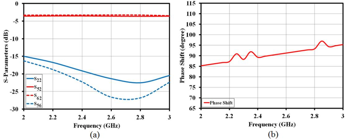
Figure 3.4: (a)  $S_{22}$ ,  $S_{52}$ ,  $S_{62}$  and  $S_{56}$  (b) phase shift of single section WPD with wide-band  $90^\circ$  phase shifter at S-band [1]
