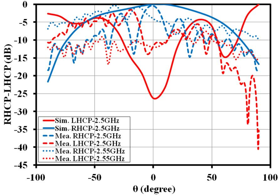
Figure 3.31: Simulated and measured RHCP-LHCP radiation patterns at S-band for  $\phi=0^\circ$  of tri-band RDRA (single port) [8]
