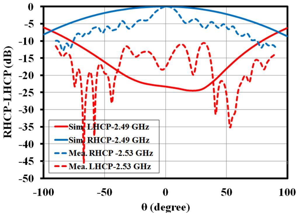
Figure 5.29: Simulated and measured RHCP-LHCP far field radiation patterns for S-band at  $\phi=0^\circ$
