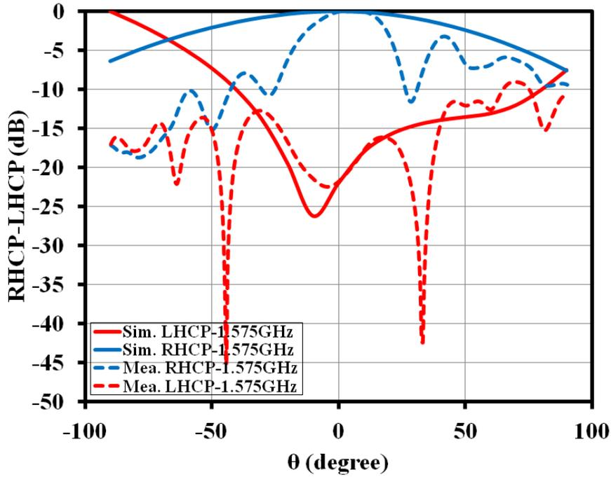
Figure 3.36: Simulated and measured RHCP-LHCP radiation patterns at L1-band for  $\phi=90^\circ$  of tri-band RDRA (single port) [8]
