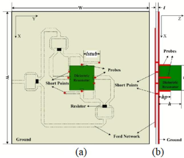
Figure 2.35: (a) Top view and (b) side view of wide-band CP RDRA with sequentially rotated feed network [55]
