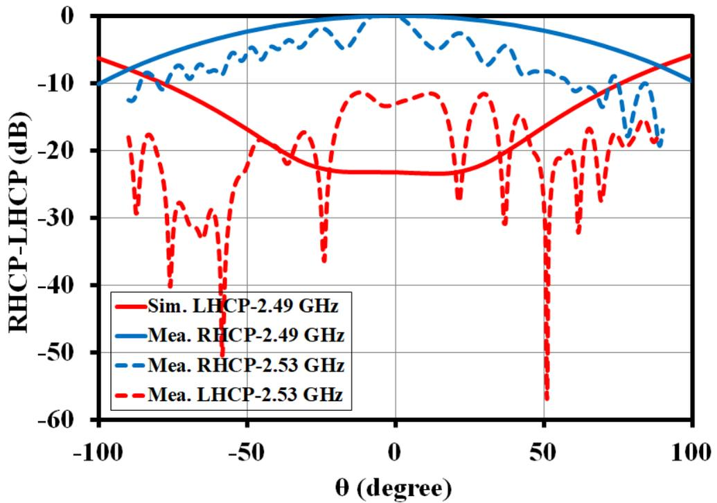
Figure 5.31: Simulated and measured RHCP-LHCP far field radiation patterns for S-band at  $\phi=90^\circ$
