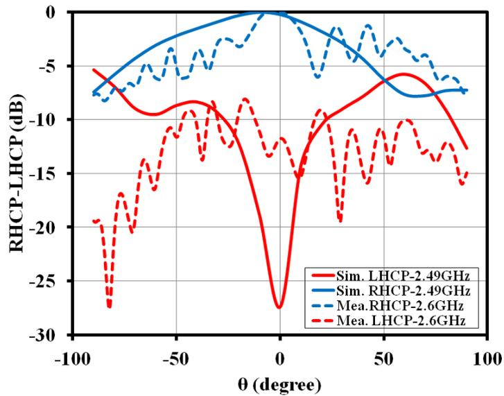
Figure 3.21: Simulated and measured RHCP-LHCP radiation patterns of tri-band RDRA at S-band for  $\phi=0^\circ$  [1]
