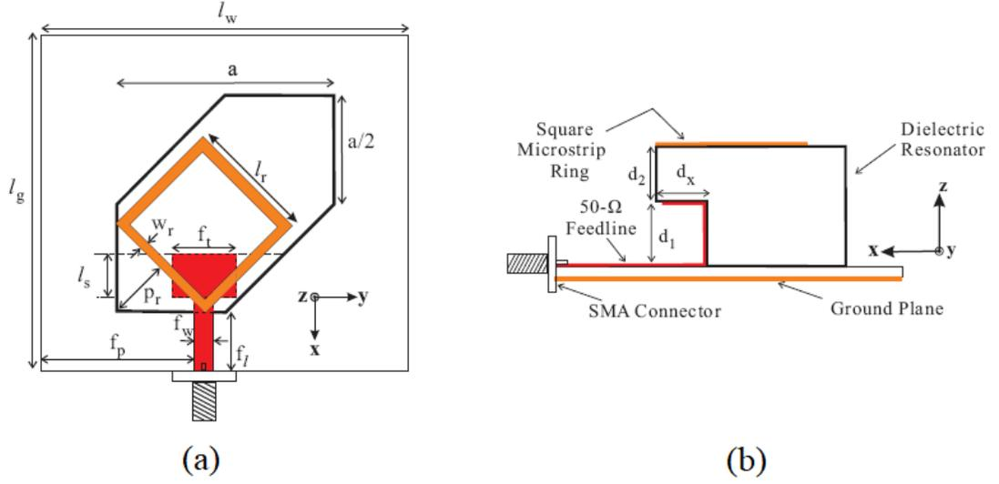
Figure 2.11: Structure of of tri-band hybrid DRA (a) top view (b) side view [11]
