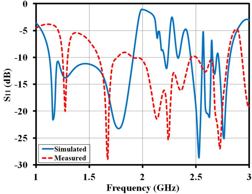
Figure 3.28: Simulated and measured  $S_{11}$  of tri-band RDRA (single port) [8]
