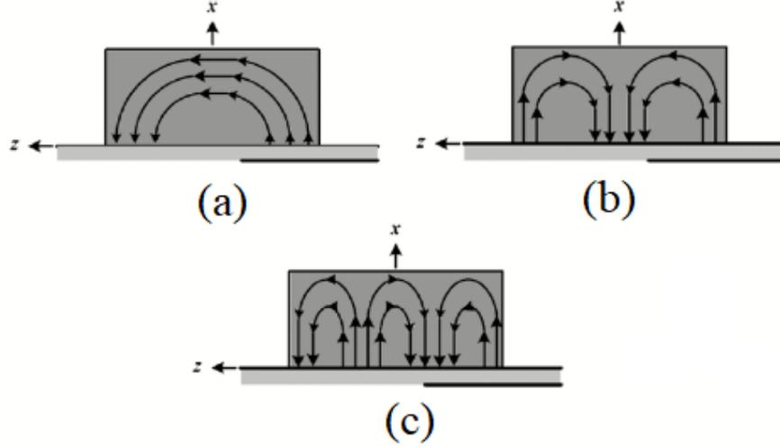
Figure 2.5: Electric field distribution of (a)  $TE_{111}^y$  mode (b)  $TE_{112}^y$  mode (c)  $TE_{113}^y$  mode of DRA [4]
