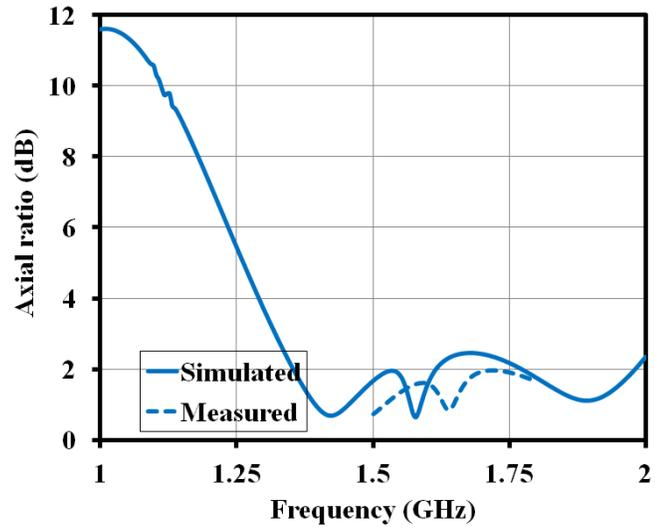
Figure 5.39: Simulated and measured axial ratio of single-band RDRA [6]
