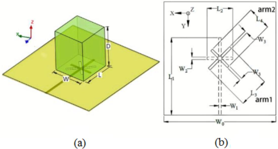
Figure 2.18: (a) 3-D view (b) top view of dual-band RDRA [18]
