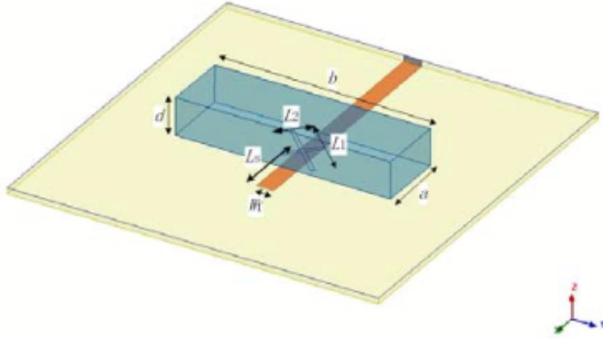
Figure 2.24: 3-D geometry of wide dual-band CP RDRA [34]
