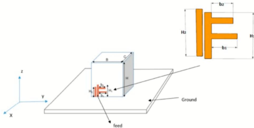
Figure 2.17: Geometry of higher order mode tri-band CP RDRA [26]
