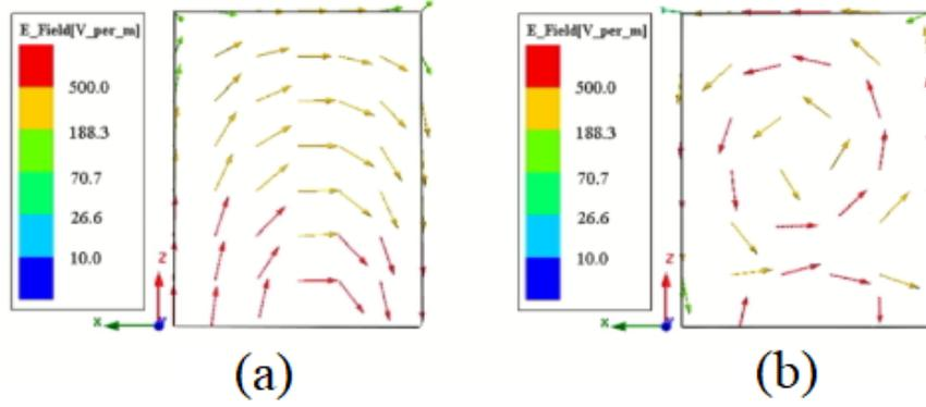
Figure 2.19: Electric field distribution of (a)  $TE_{111}$  mode (b)  $TE_{113}$  mode of dual-band RDRA [18]
