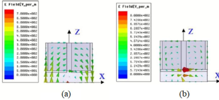
Figure 2.21: Electric field distribution of (a) quasi- $TE_{111}$  mode (b) quasi- $TE_{113}$  mode of dual-band RDRA [28]
