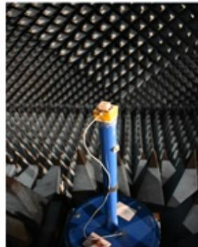
Figure 5.9: Photograph of fabricated single-band RDRA for test and measurement in the anechoic chamber
