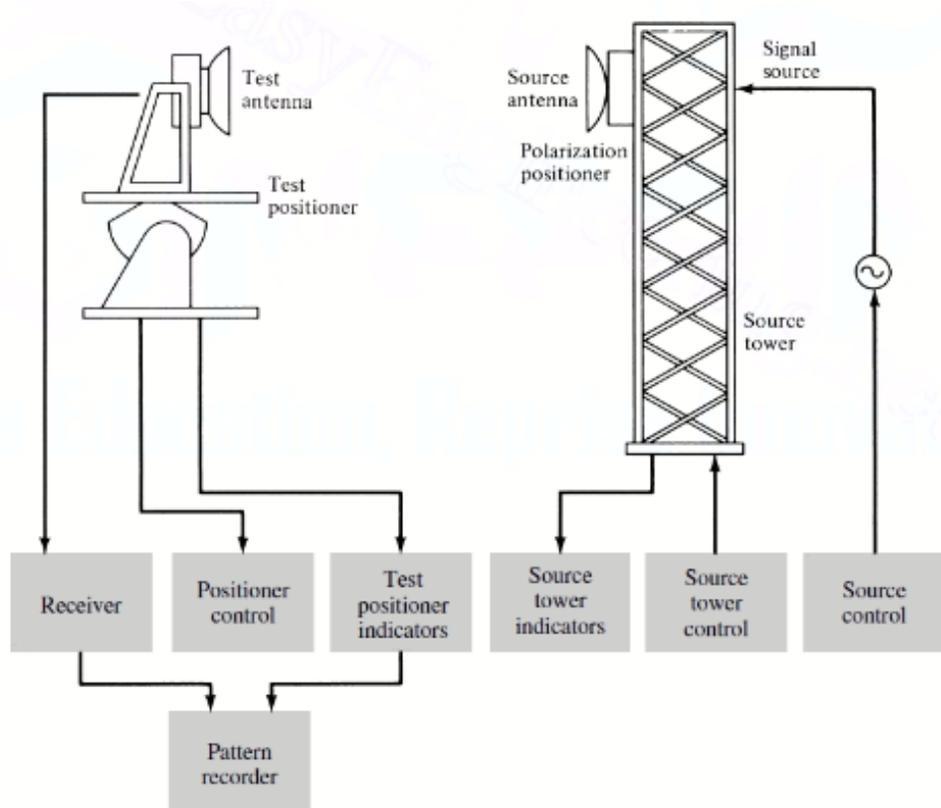
Figure A.1: Measurement system for CP RDRAs in the anechoic chamber [1]
