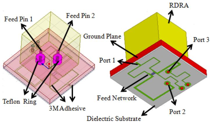
Figure 5.12: 3-D geometries of single-band RDRA [6]
