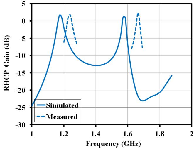
Figure 4.14: Simulated and measured RHCP gain at L5 and L1-bands of dual-band RDRA
