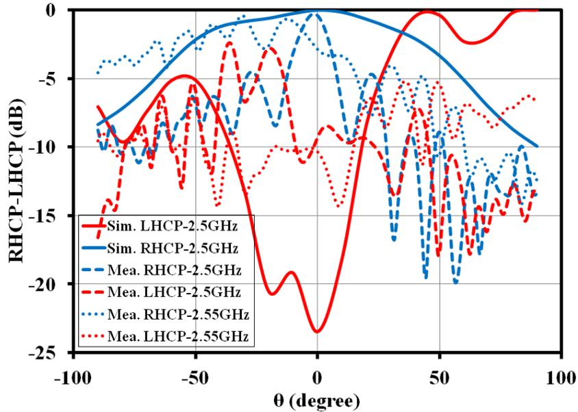
Figure 3.34: Simulated and measured RHCP-LHCP radiation patterns at S-band for  $\phi=45^\circ$  of tri-band RDRA (single port) [8]
