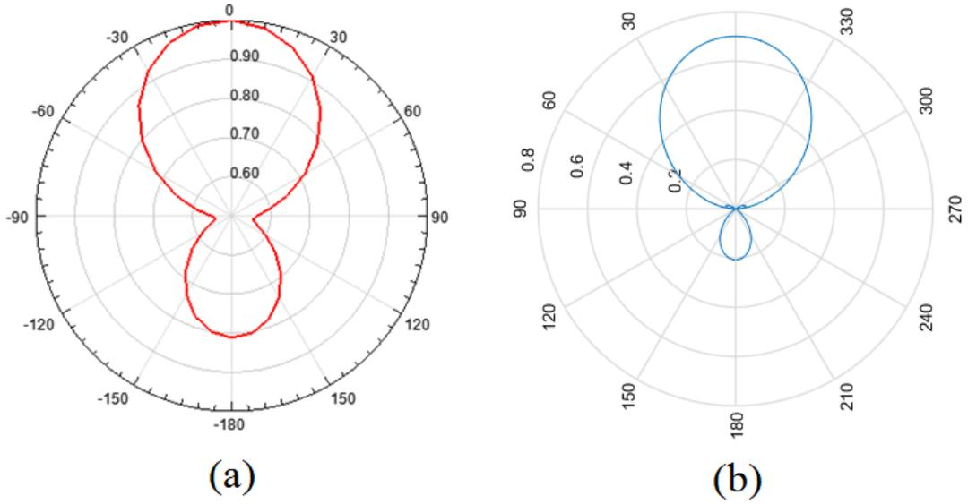
Figure 6.13: (a) Normalized electric field radiation patterns at 1.176 GHz of single-band RDRA using reference [3] (b) Normalized electric field radiation patterns at 1.176 GHz of single-band RDRA using MoM
