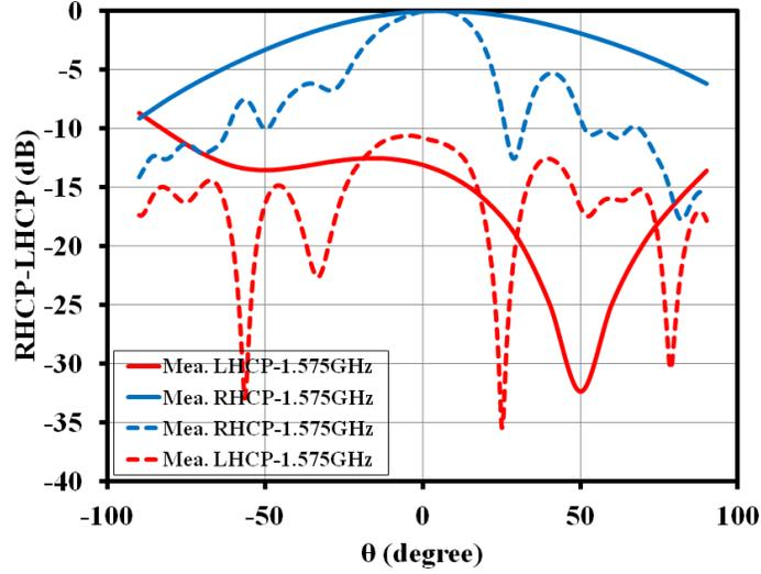
Figure 3.26: Simulated and measured RHCP-LHCP radiation patterns of tri-band RDRA at L1-band for  $\phi=90^\circ$  [1]
