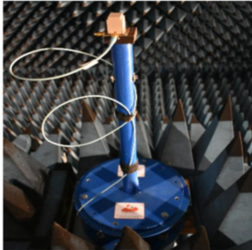
Figure 3.8: Photograph of fabricated triband RDRA with bakelite support, mounting fixture and fixure pipe in anechoic chamber [1]
