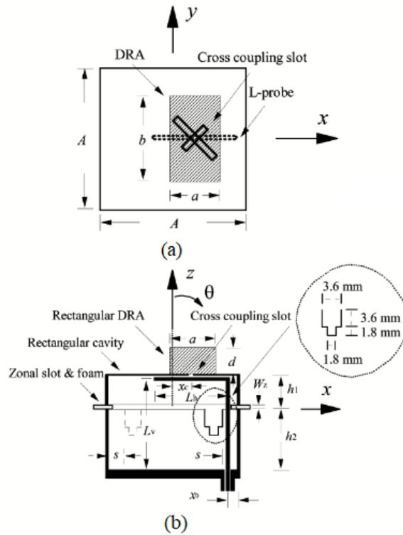
Figure 2.23: (a) Top view and (b) front view of dual-band zonal-slot hybrid DRA [33]
