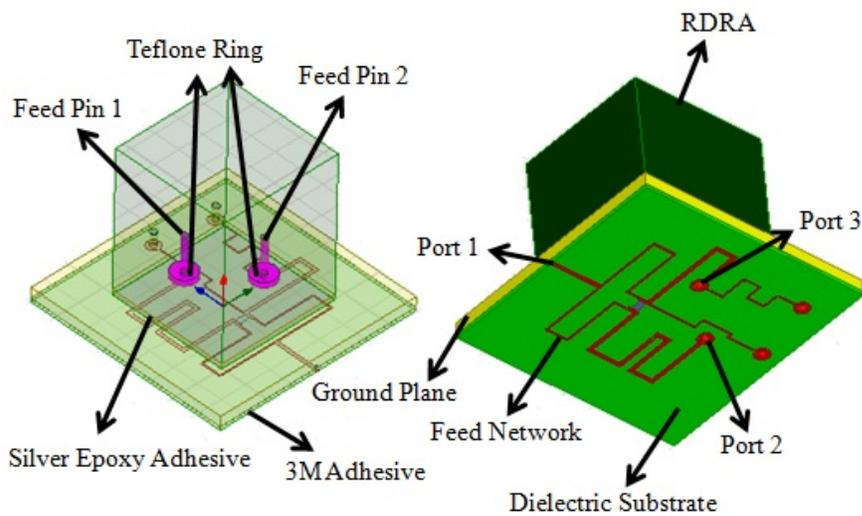
Figure 5.21: 3-D geometries of single-band RDRA [6]
