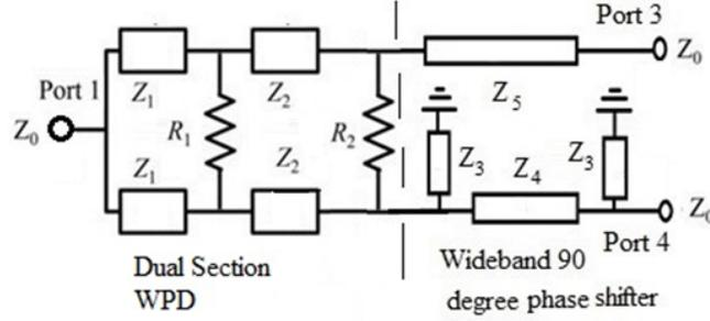
Figure 4.4: Dual-section WPD with wide-band  $90^\circ$  phase shifter [1]
