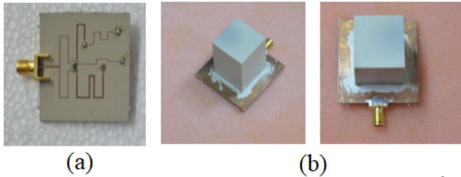
Figure 5.26: Photograph of (a) bottom view (b) 3-D geometries views of fabricated single-band RDRA [6]
