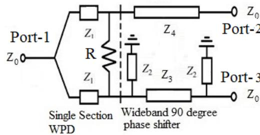
Figure 5.4: Feed network of WPD with wide-band  $90^\circ$  phase shifter [1, 3, 4]
