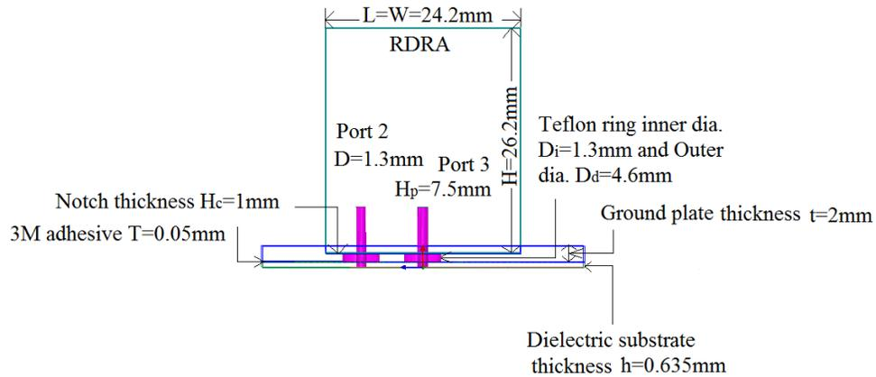
Figure 4.1: Front view of dual-band RDRA [1]
