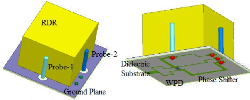
Figure 5.3: 3-D geometry views of single-band RDRA
