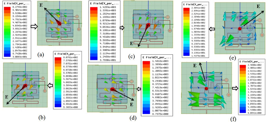
Figure 3.12: Electric field distribution of tri-band RDRA (a) 1.176 GHz with respect to  $0^\circ$  (b) 1.176 GHz with respect to  $90^\circ$  (c) 1.575 GHz with respect to  $0^\circ$  (d) 1.575 GHz with respect to  $90^\circ$  (e) 2.49 GHz with respect to  $0^\circ$  (f) 2.49 GHz with respect to  $90^\circ$  [8]
