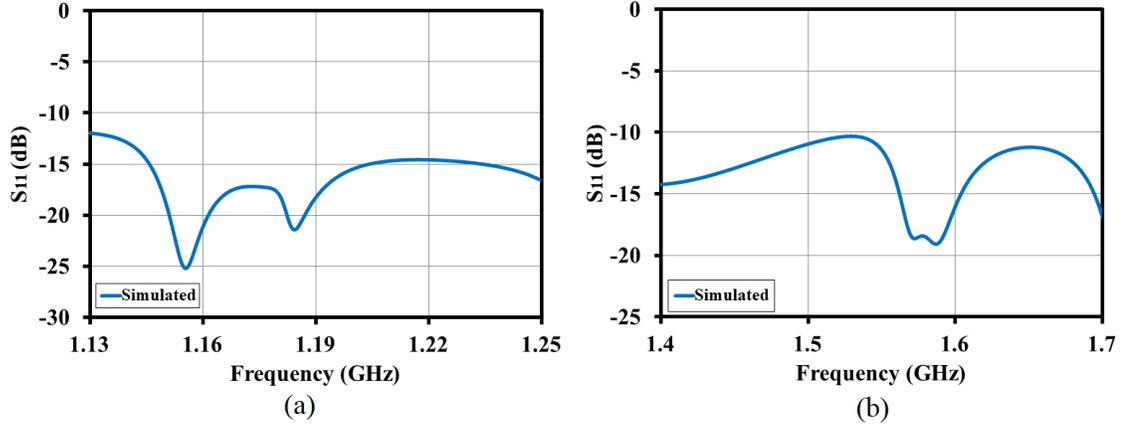
Figure 6.3: Simulated  $S_{11}$  of (a) L5-band RDRA and (b) L1-band RDRA [4]
