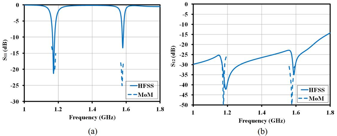
Figure 6.5: (a)  $S_{11}$  and (b)  $S_{12}$  of dual-band RDRA using reference [3] and MoM
