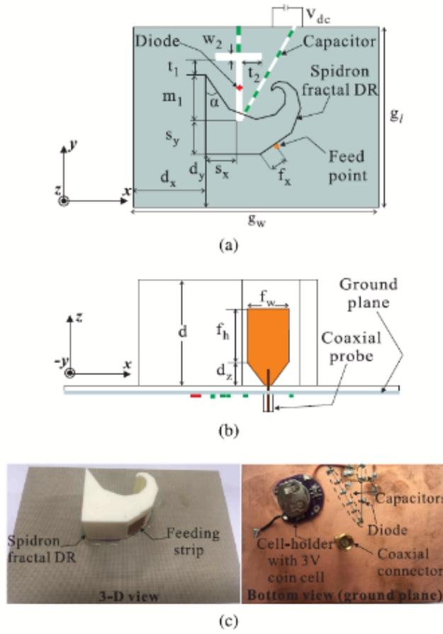
Figure 2.27: (a) Top view (b) side view (c) photograph of fabricated reconfigurable dual-/tri-band CP DRA [37]
