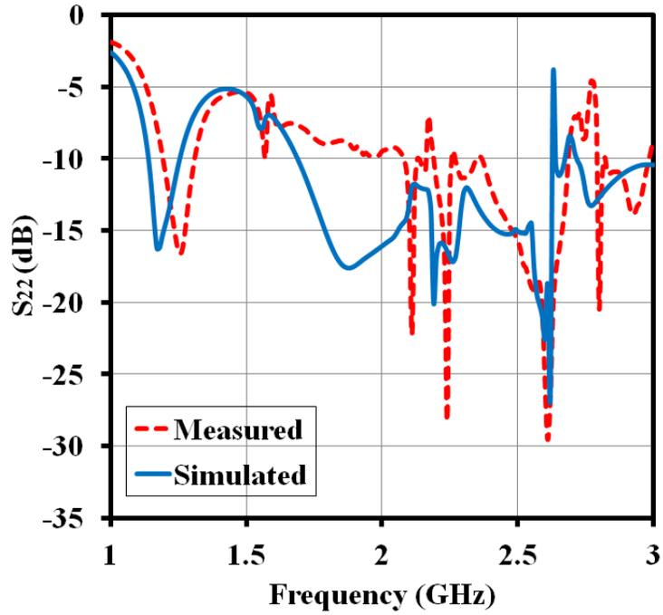
Figure 3.16: Simulated and measured  $S_{22}$  of tri-band RDRA (two port) [1]
