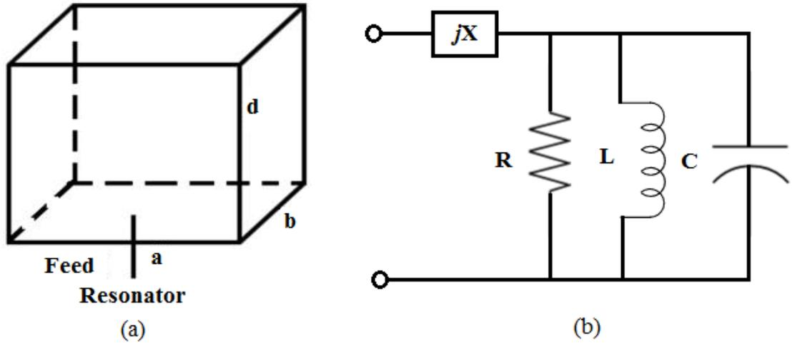
Figure 1.1: (a) Ceramic dielectric resonator antenna with dimensions of a, b and d (b) DRA equivalent RLC circuit [9]
