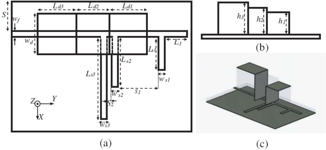
Figure 2.16: Geometry of tri-band RDRA (a) top view (b) side view (c) metalized plates [21]
