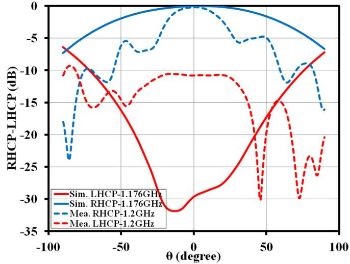
Figure 3.22: Simulated and measured RHCP-LHCP radiation patterns of triband RDRA at L5-band for  $\phi=45^\circ$  [1]
