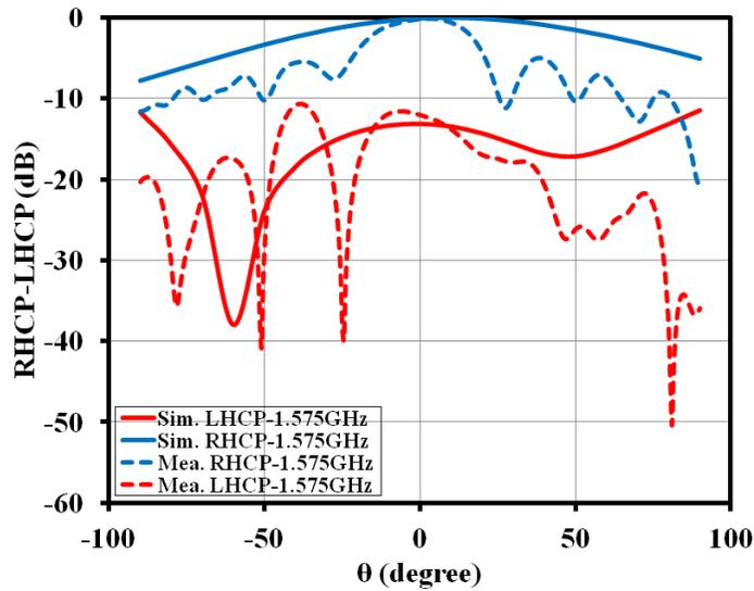
Figure 3.23: Simulated and measured RHCP-LHCP radiation patterns of tri-band RDRA at L1-band for  $\phi=45^\circ$  [1]
