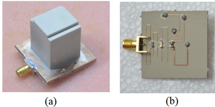
Figure 3.13: (a) 3-D view and (b) bottom view of fabricated tri-band RDRA [8]
