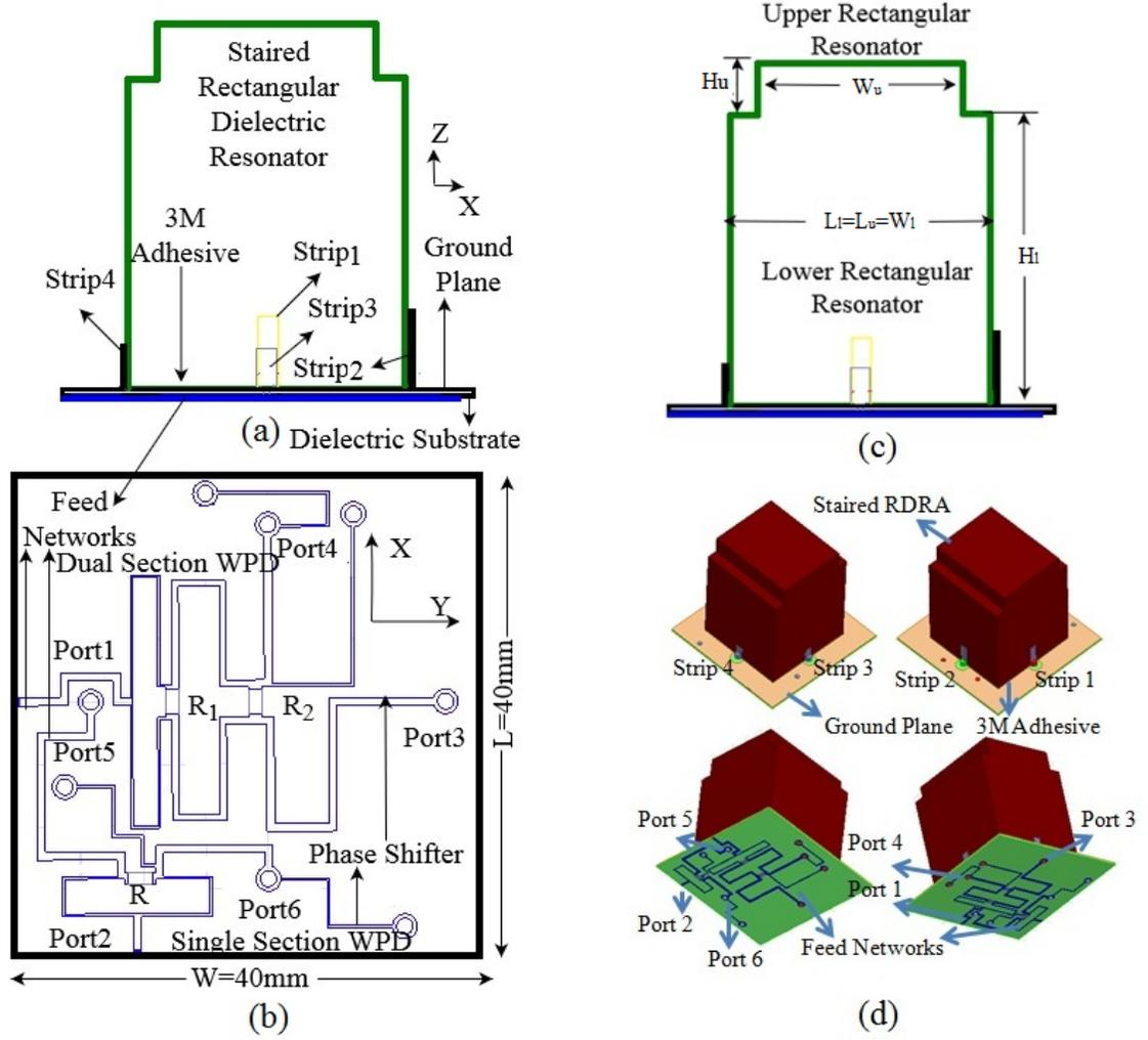
Figure 3.1: Geometry of compact tri-band RDRA with finite ground plane
