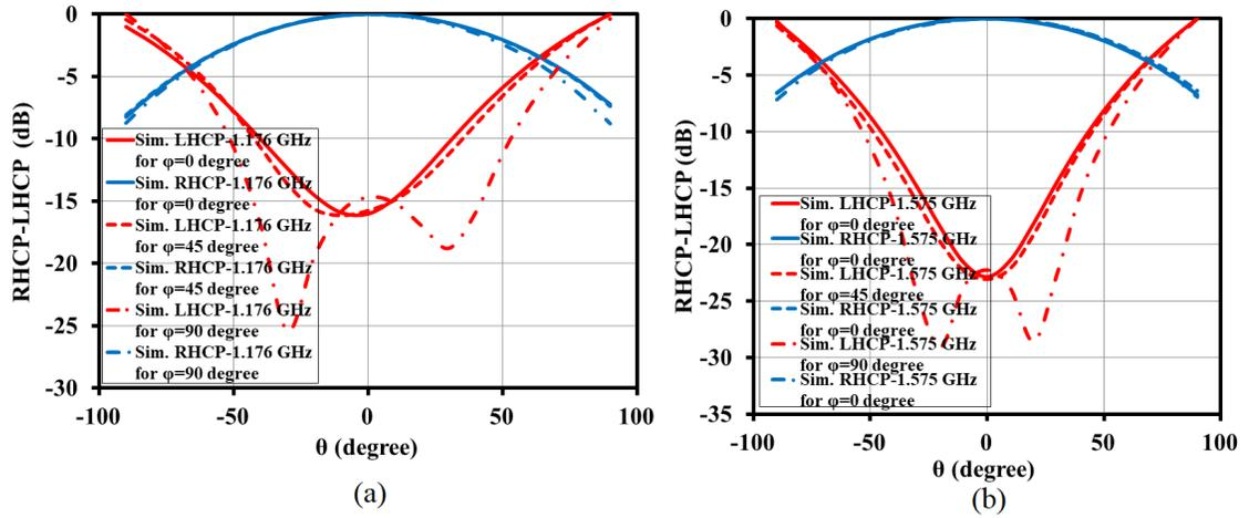
Figure 6.4: Simulated RHCP-LHCP far field radiation patterns of (a) L5-band RDRA and (b) L1-band RDRA [4]
