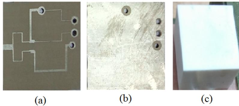
Figure 5.8: Photographs of single-band RDRA parts (a) bottom view of dielectric substrate (b) top view of dielectric substrate (c) rectangular dielectric resonator [1]
