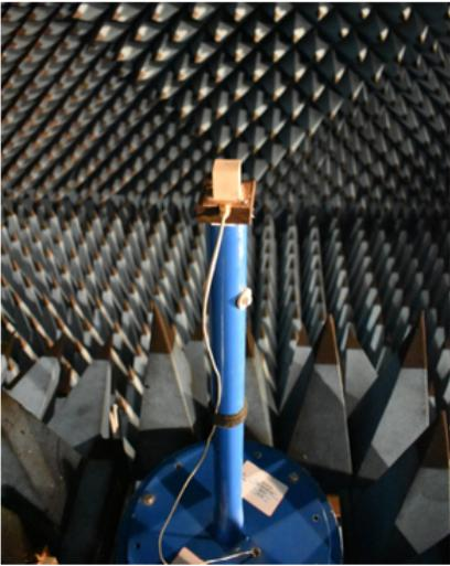
Figure 4.9: Testing of fabricated dual-band RDRA in the anechoic chamber
