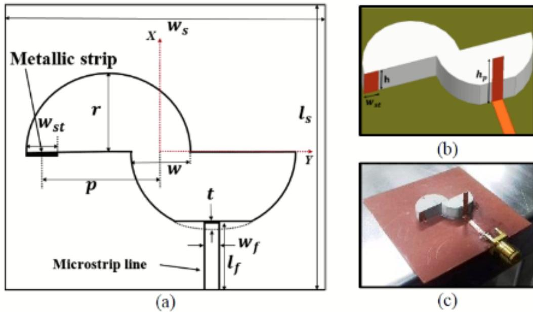
Figure 2.26: (a) Configuration of multi-band CP DRA (b) feeding patch applied at DR surface (c) photograph of fabricated antenna [36]
