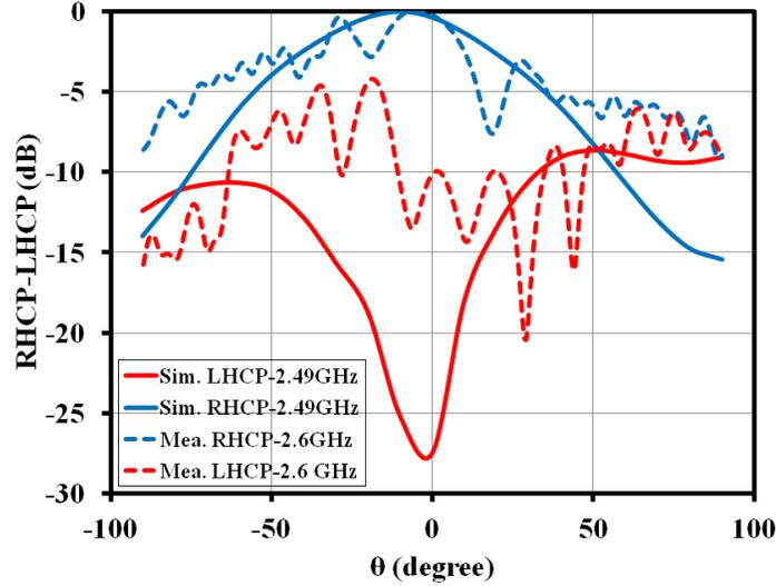
Figure 3.24: Simulated and measured RHCP-LHCP radiation patterns of tri-band RDRA at S-band for  $\phi=45^\circ$  [1]
