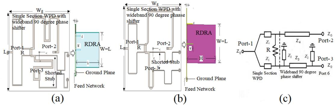
Figure 6.1: Geometries of single-band RDRAs (a) L5-band RDR (b) L1-band RDR and (c) schematic of feed network [4]
