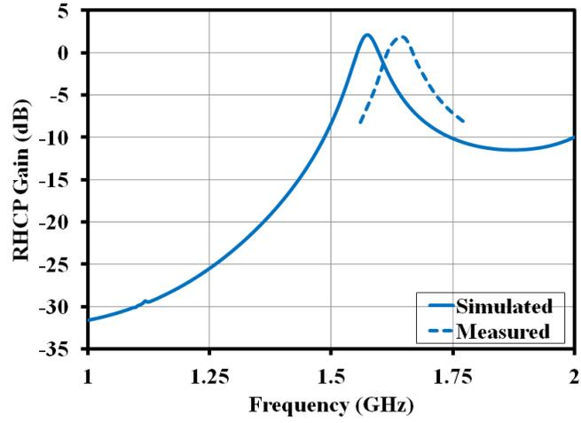
Figure 5.38: Simulated and measured RHCP gain of single-band RDRA [6]
