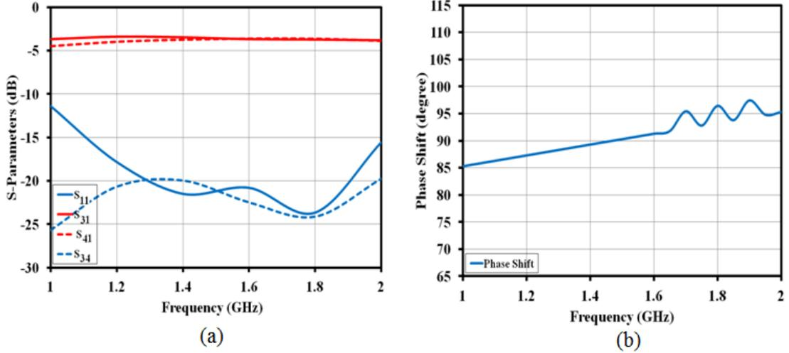
Figure 3.3: (a)  $S_{11}$ ,  $S_{31}$ ,  $S_{41}$  and  $S_{34}$  (b) phase shift of dual-section WPD with wide-band  $90^\circ$  phase shifter at L5- and L1-band [1]
