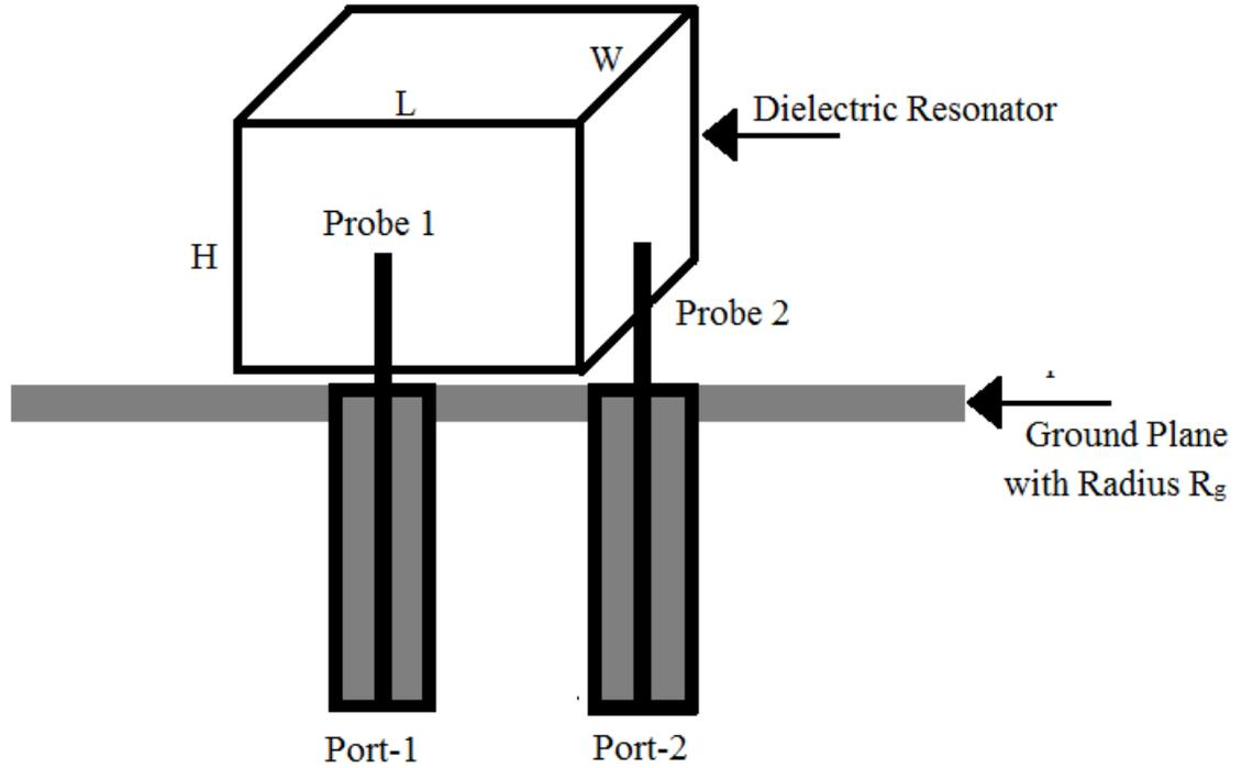
Figure 6.2: Geometry of CP dual and single-band RDRAs
