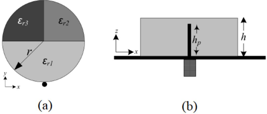
Figure 2.15: Structure of tri-band CDRA using varying permittivity in  $\phi$ -direction (a) top view (b) front view [19]
