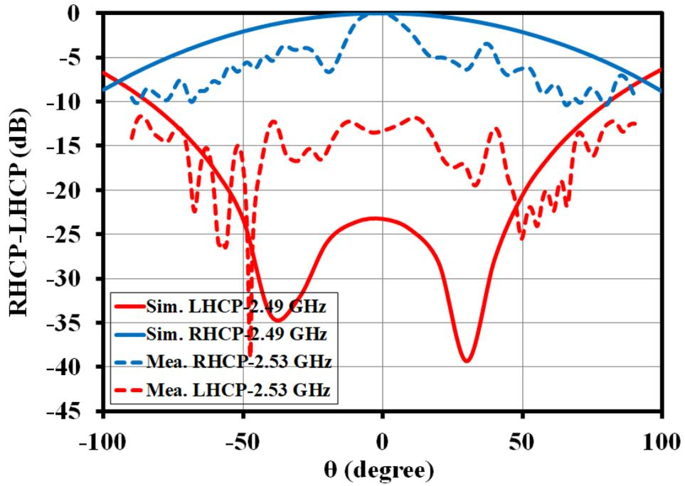
Figure 5.30: Simulated and measured RHCP-LHCP far field radiation patterns for S-band at  $\phi=45^\circ$
