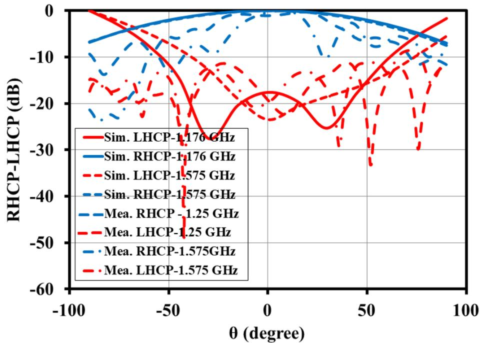
Figure 4.13: Simulated and measured RHCP-LHCP radiation patterns at L5 and L1-band of dual-band DRA for  $\phi=90^\circ$
