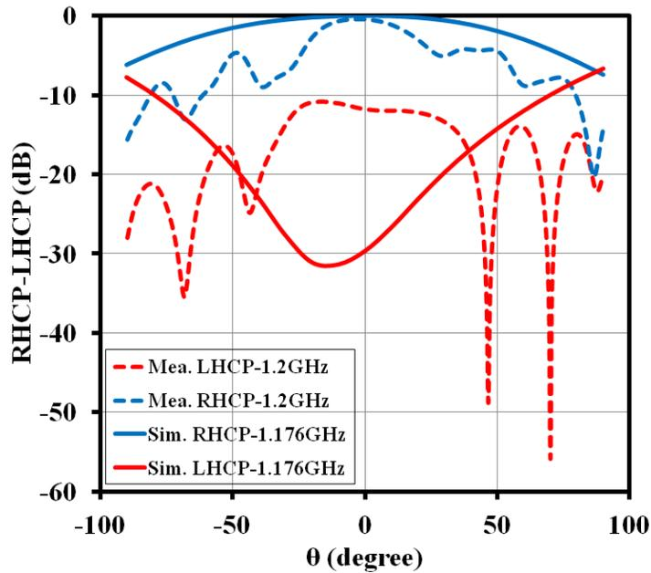
Figure 3.19: Simulated and measured RHCP-LHCP radiation patterns of tri-band RDRA at L5-band for  $\phi=0^\circ$  [1]
