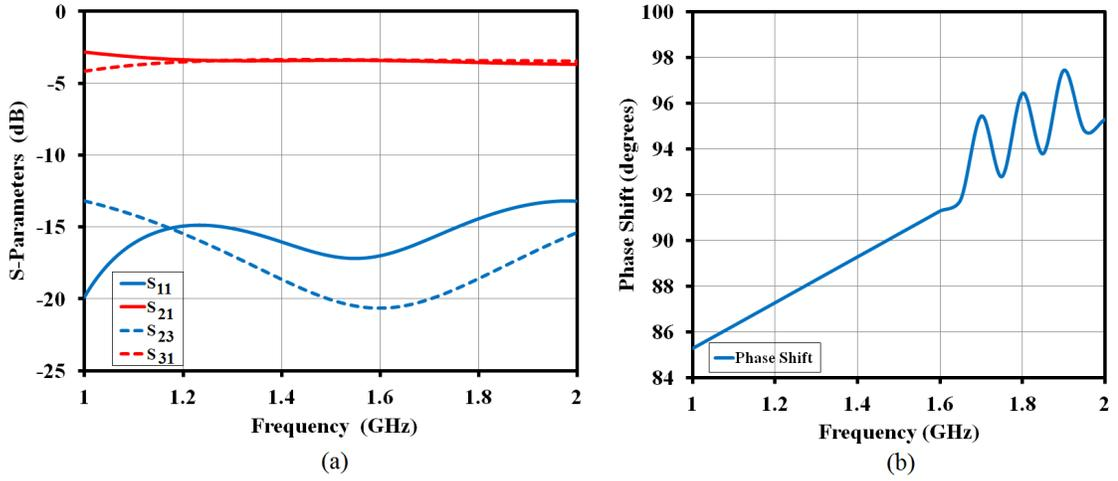
Figure 5.14: (a) S-parameters ( $S_{11}$ ,  $S_{21}$ ,  $S_{31}$ ,  $S_{23}$ )
