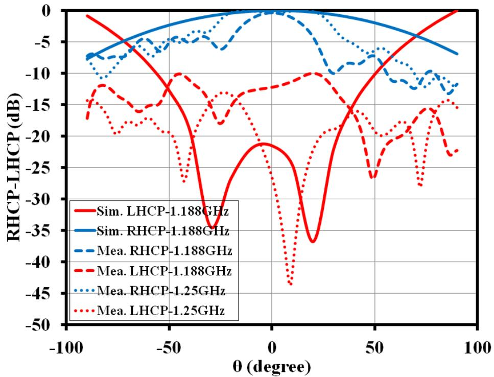
Figure 5.43: Simulated and measured RHCP-LHCP far field radiation patterns for L5-band at  $\phi=90^\circ$  [6]
