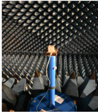
Figure 5.27: Photograph of fabricated single-band RDRA for test and measurement in the anechoic chamber
