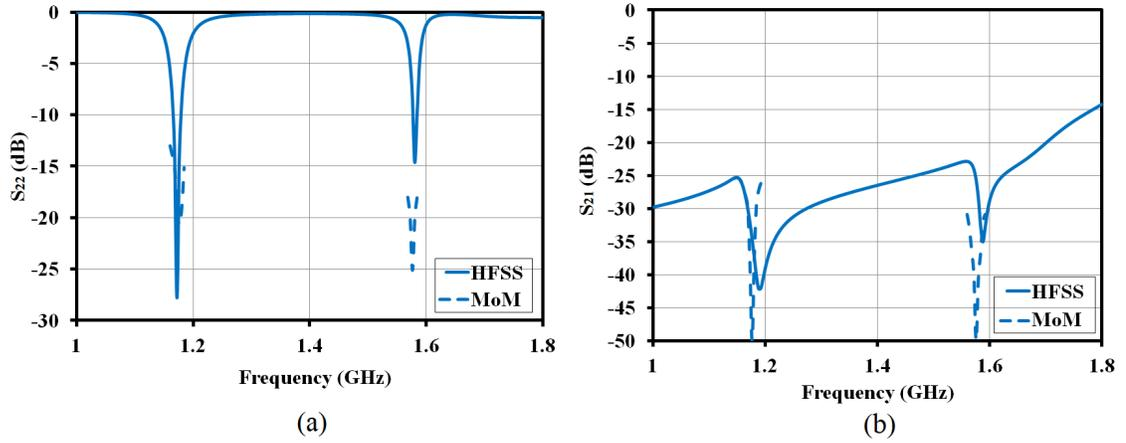
Figure 6.6: (a)  $S_{22}$  and (b)  $S_{21}$  of dual-band RDRA using reference [3] and MoM
