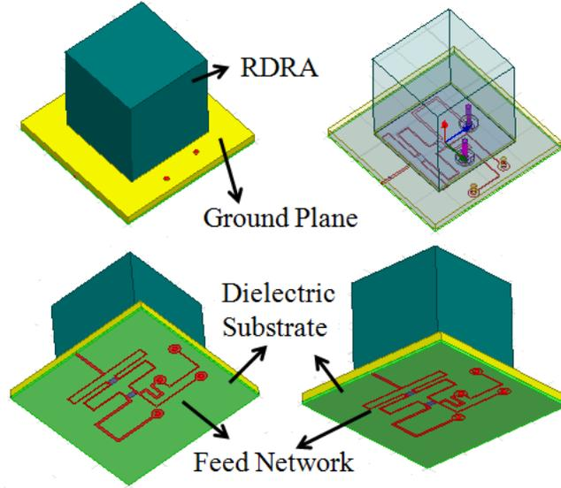
Figure 4.3: 3-D geometry views of dual-band RDRA [1]
