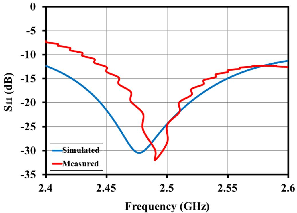
Figure 5.28: Simulated and measured  $S_{11}$  of single-band RDRA
