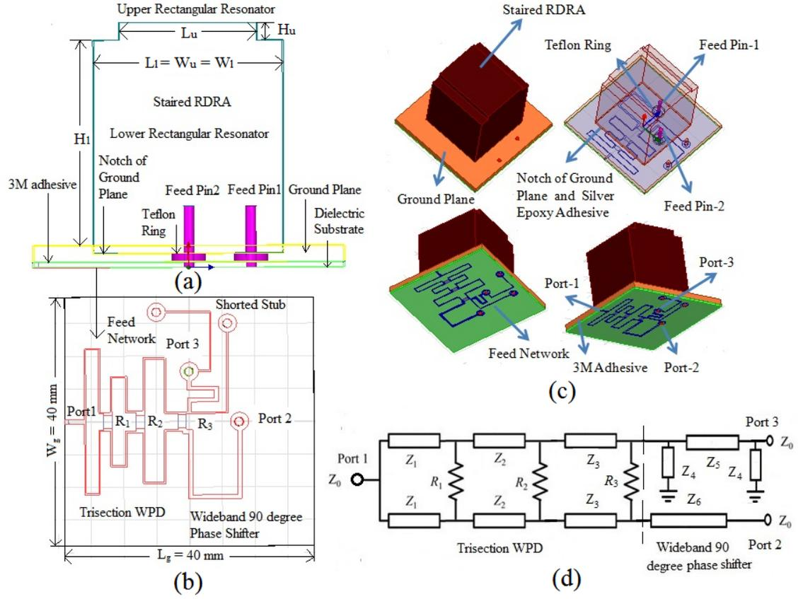
Figure 3.9: Configuration of miniaturized tri-band CP RDRA
