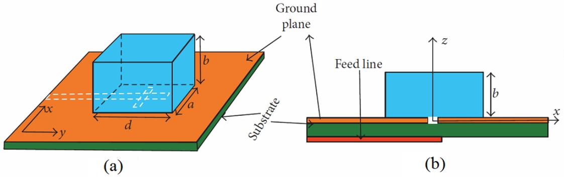
Figure 2.4: (a) 3-D cross-sectional view of RDRA (b) aperture-fed RDRA [1]
