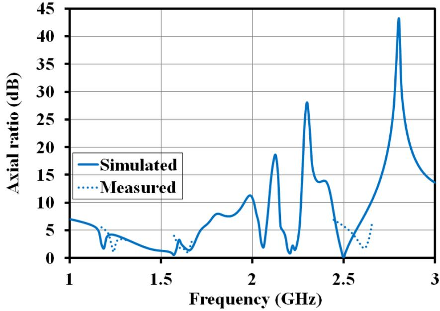
Figure 3.39: Simulated and measured axial ratio of tri-band RDRA (single port)
